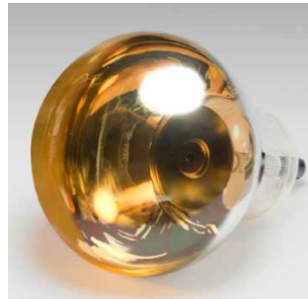
Hybrid Photo-Detector (HPD)
