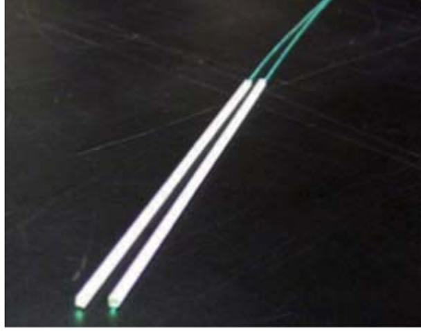
Figure 5.15: Fiber scintillator for charge division study to define the incident position with a good precision
