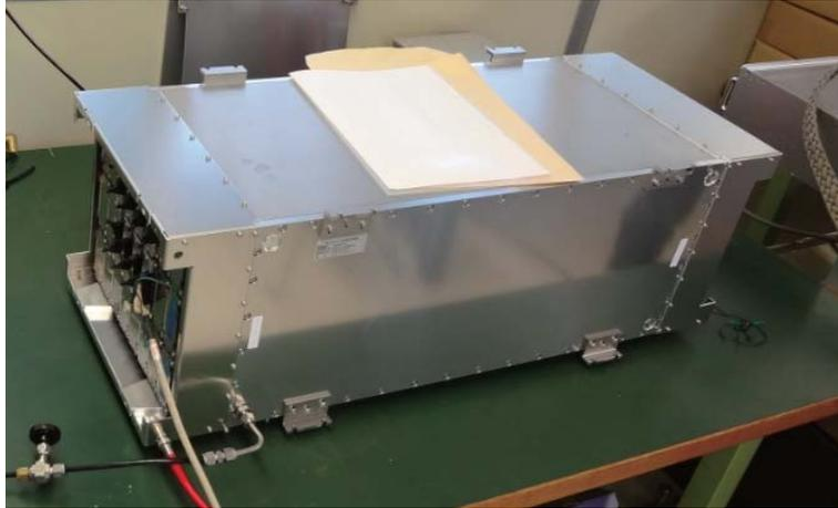
Figure 4.5: MTP (size: 865mm  $\times$  284mm  $\times$  330mm, 75kg)
