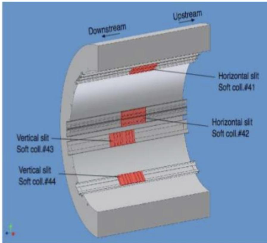
Figure 3.13: Places where Pb collimators were installed.
