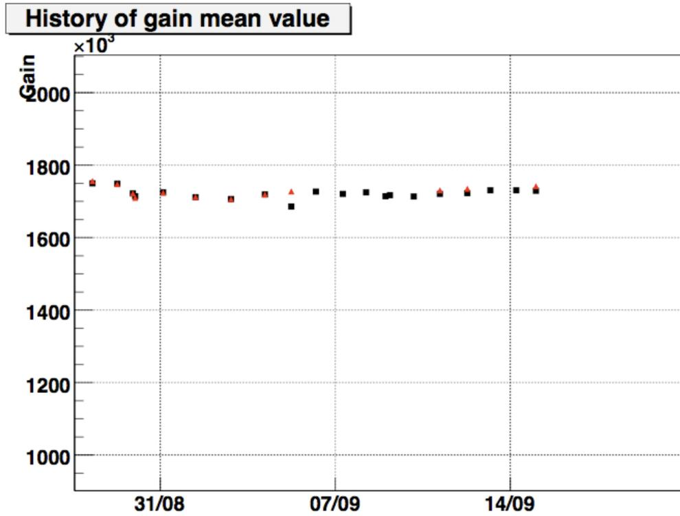
Figure 3.4: History of gain. Red and black dots represent values from trigger and DRS data respectively.
