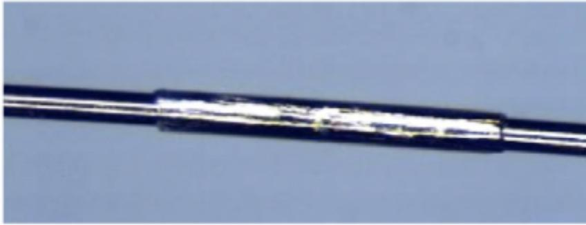
Figure 3.5: Alpha source on a wire. Length of the source is 1mm, and diameter of the wire is  $100\mu\text{m}$ .
