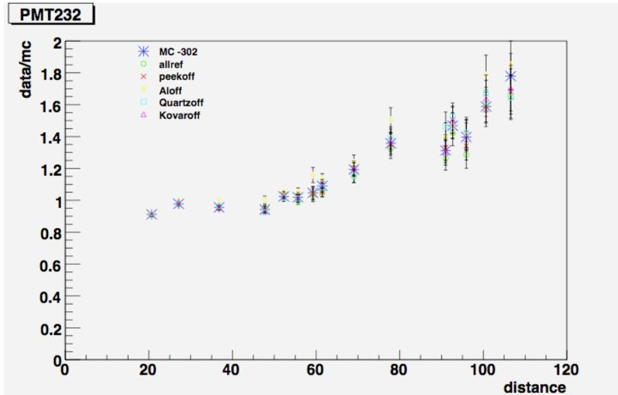
Figure 4.7: Data/MC ratio in relation to distance. Several simulations were done by turning off reflection on each material.
