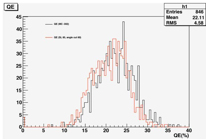
Figure 5.1: Distribution of QE with old simulation and QE with longer scattering length (85cm) and lower incidence angle cut ( $60^\circ$ )
