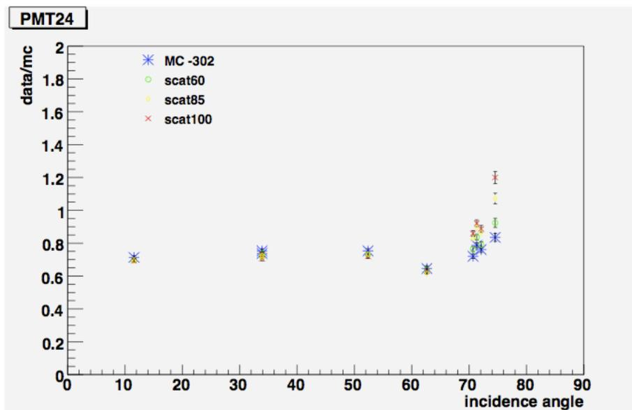
Figure 4.6: Data/MC ratio in relation to incidence angle. Several simulations were made by changing the scattering length from 45cm to 60cm, 85cm, 100cm.
