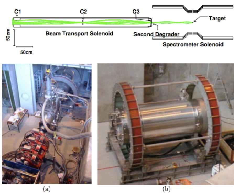
Figure 2.4: (a) Muon beam carried to target inside the COBRA magnet by the Beam Transport Solenoid (BTS). (b) COBRA magnet.
