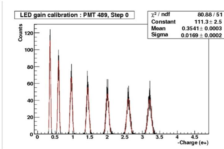
Figure 3.2: Spectrum of charge of a PMT. Intensity of LEDs are changed in 7 steps.
