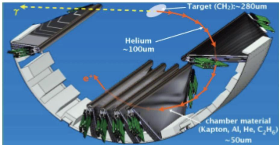
Figure 2.6: Schematic view of the drift chamber system.
