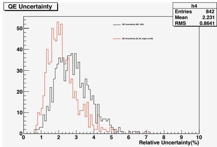
Figure 5.2: Error of QE measurement with old simulation and error of QE measurement with longer scattering length (85cm) and lower incidence angle cut (60°)
