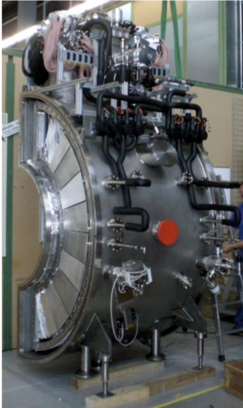
Figure 2.22: A picture of liquid xenon detector with the cryostat installed.
