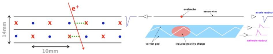
Figure 2.7: Cross view of the drift chamber and reading from Vernier pads.
