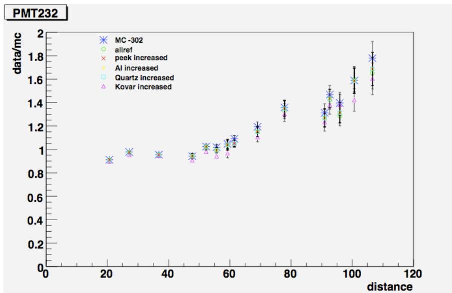
Figure 4.9: Data/MC ratio in relation to distance. Several simulations were done by increasing reflection on each material.
