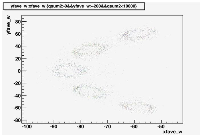
Figure 3.8: Weighted mean position of PMT outputs in alpha events in liquid xenon.
