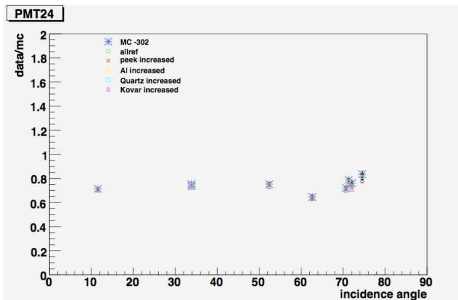
Figure 4.10: Data/MC ratio in relation to incidence angle. Several simulations were done by increasing reflection on each material.
