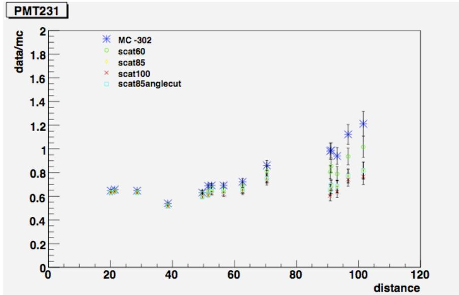
Figure 4.5: Data/MC ratio in relation to distance. Several simulations were made by changing the scattering length from 45cm to 60cm, 85cm, 100cm.
