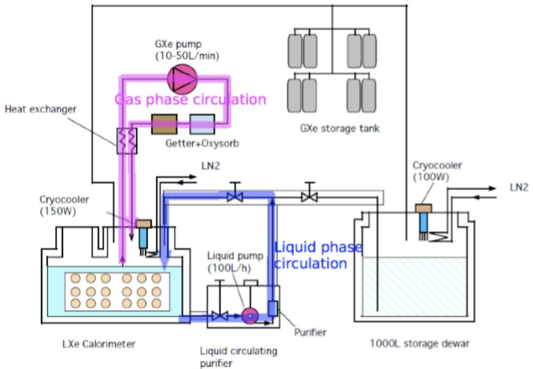
Figure 2.20: Schematic view of the xenon line.
