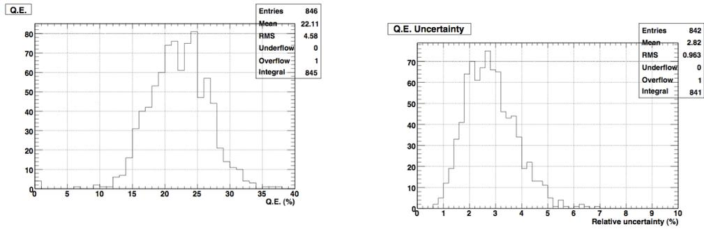
Figure 3.11: (a)Distribution of measured QE values. (b)Relative errors of QE measurement.
