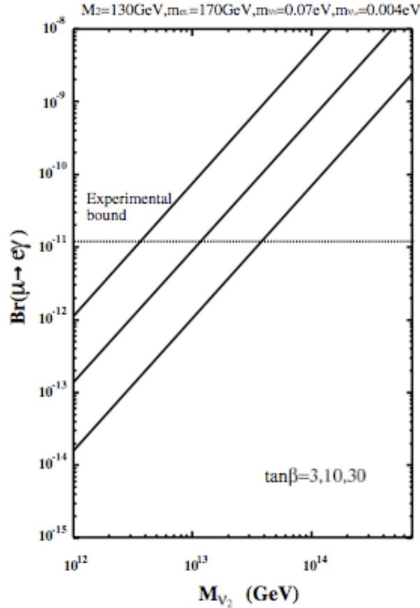
Figure 1.3: Branching ratio of  $\mu^+ \rightarrow e^+\gamma$  according to MSSMRN in the case of MSW large angle solution. The three lines represent where  $\tan\beta = 30, 10, 3$  respectively.
