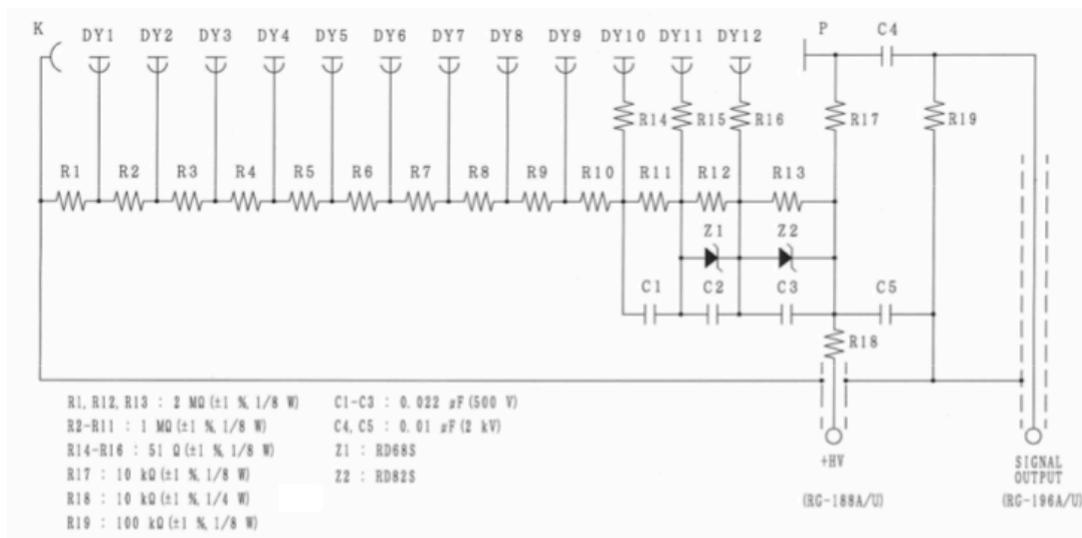
Figure 2.14: Circuit diagram of R9288.
