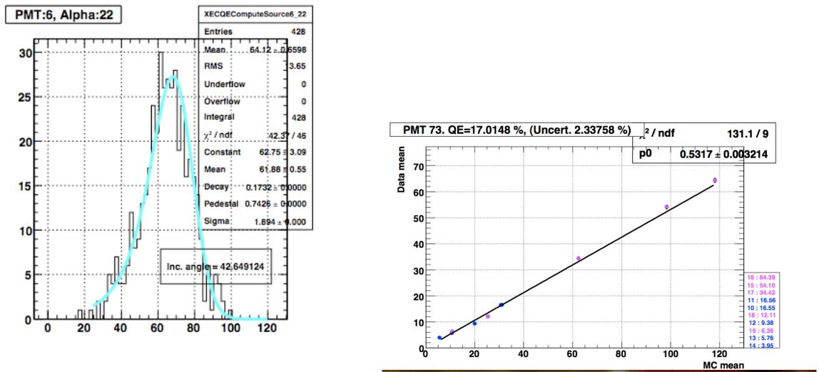
Figure 3.10: (a) An example of charge spectrum from a given alpha source observed by a PMT. (b) The mean value of the fitting function is compared with simulation. QE can be estimated from the slope.
