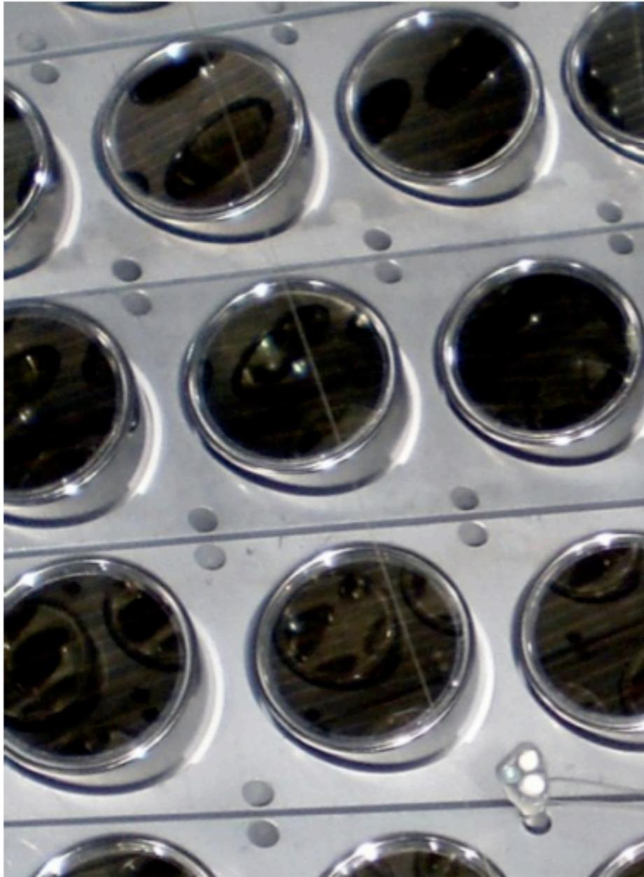
Figure 3.7: Alpha source wire and LED bundle.
