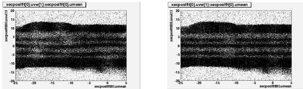
Figure 3.14: 2D vertex distribution with horizontal lead collimator before and after QE correction.
