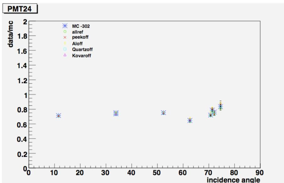
Figure 4.8: Data/MC ratio in relation to incidence angle. Several simulations were done by turning off reflection on each material.
