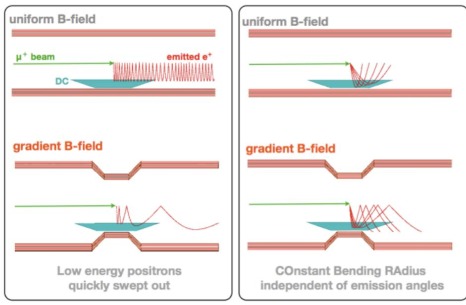
Figure 2.5: Comparison between uniform and gradient magnetic field.
