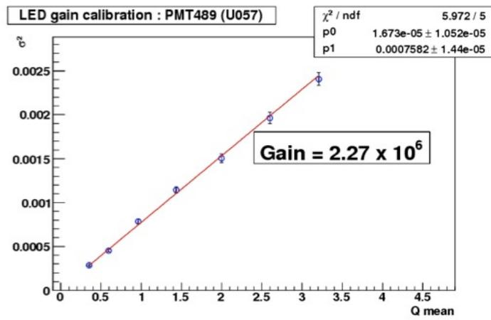
Figure 3.3: Mean and  $\sigma^2$  of fitted Gaussian functions. Gain can be estimated from the slope of the plot.
