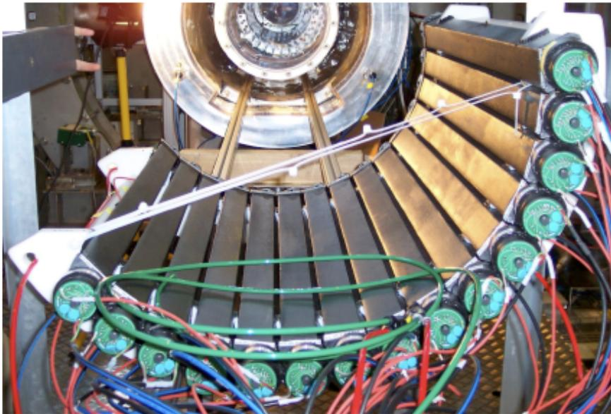
Figure 2.8: A picture of timing counters ( $\phi$ -measuring counters).
