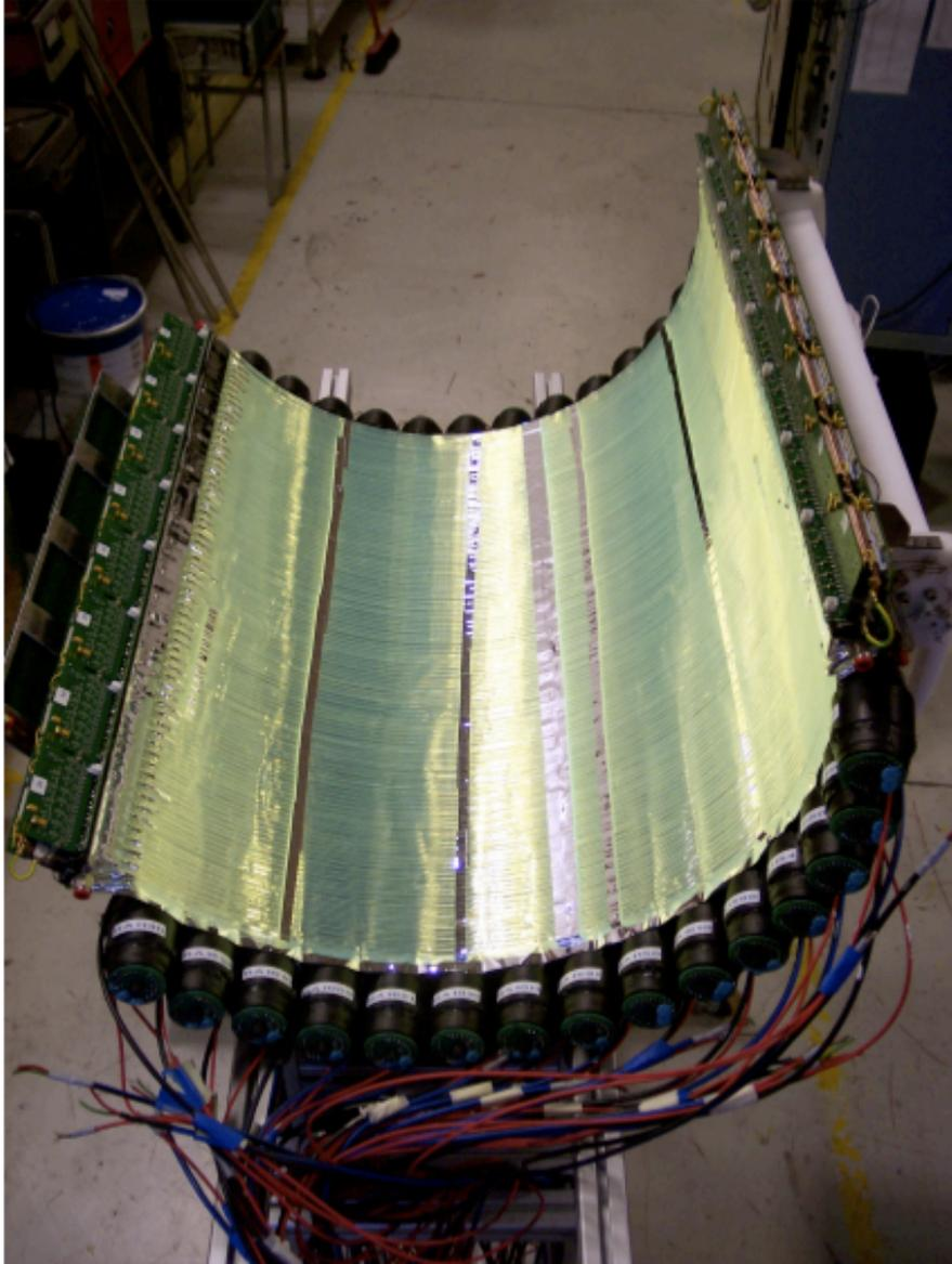
Figure 2.9: A picture of timing counters ( $z$ -measuring counters). 256 curved scintillators are put on top of  $\phi$ -measuring counters. Also seen are the attached readout cards.
