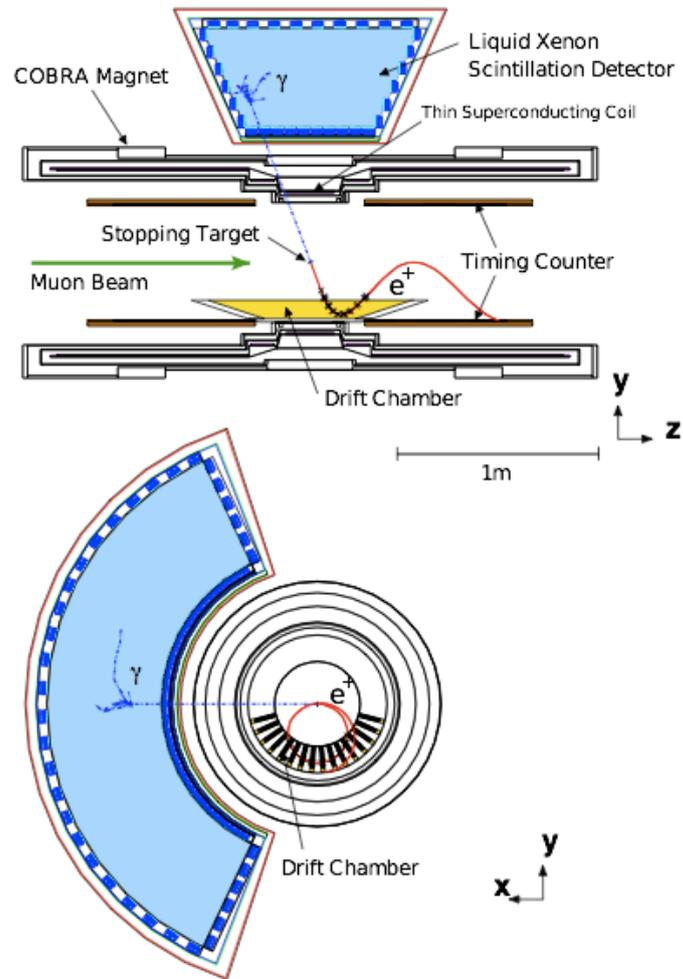
Figure 2.2: Schematic view of MEG detectors
