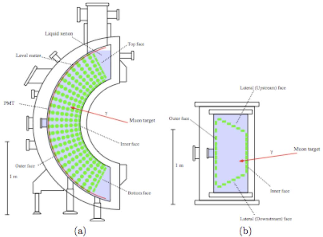
Figure 2.10: Schematic view of the MEG gamma ray detector. (a) Side view. (b) Top view.
