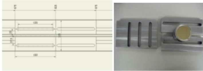
Figure 3.12: Left: geometry of Pb collimator with three horizontal slits; Right: Pb collimators with vertical and horizontal slits.
