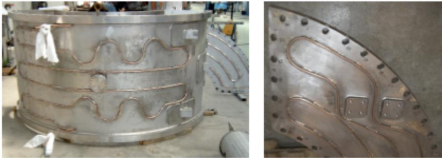
Figure 2.19: Liquid nitrogen pipe attached on inner vessel.
