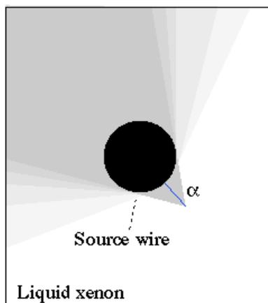
Figure 3.9: Alpha particle and the wire. Diameter of the wire is  $100 \mu\text{m}$  and the range of alpha particle in liquid xenon is about  $40 \mu\text{m}$ .
