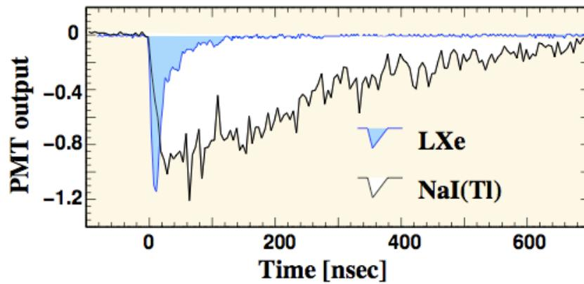
Figure 2.11: Typical waveforms of LXe and NaI(Tl) from 320keV  $\gamma$  rays. It is clear that liquid xenon has a much faster response compared to NaI.
