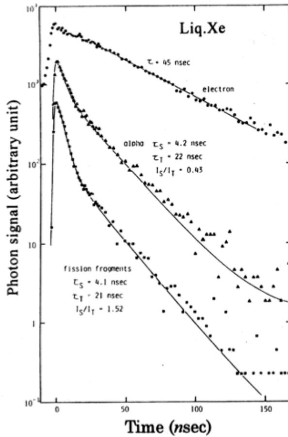
Figure 2.12: Signal of liquid xenon scintillation.
