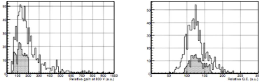
Figure 2.15: Measured gain and QE. Hatched part is PMTs used in inner face.
