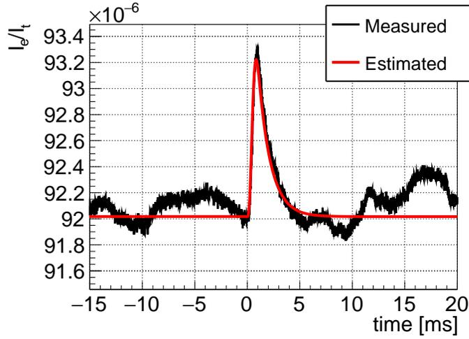
Figure 4.9: An example of the parameter estimation. Black line: Measured sign averaged ellipticity. Red line: Estimated signal.
