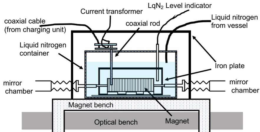
Figure 3.39: Schematic of the magnet system. On the magnet bench, the liquid container is placed. A magnet is inside the container. The magnet is surrounded by the double iron plate. A coaxial cable, a liquid nitrogen level indicator, and a current transformer are also installed.
