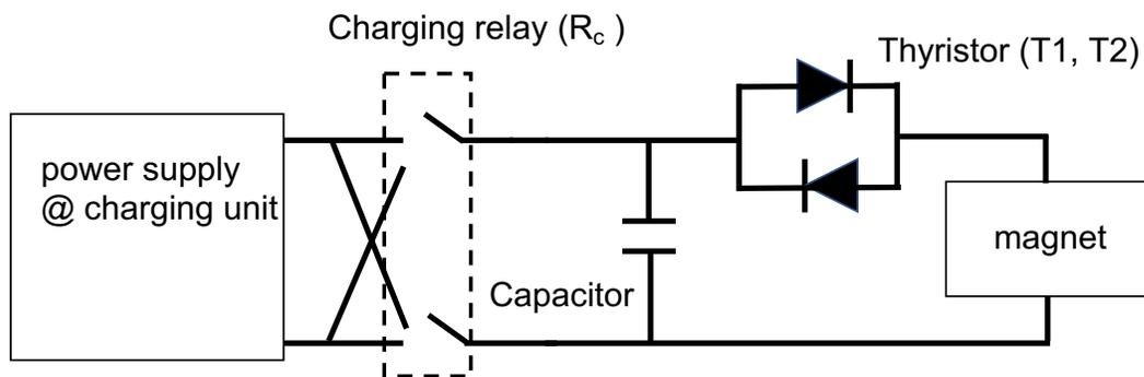
Figure C.2: Schematic view of the charging unit. The unit has 2 switches. One is the charging relay ( $R_c$ ) to control the charging to the capacitor. The other is thyristors ( $T_1$ ,  $T_2$ ) to control the discharge to the magnet.
