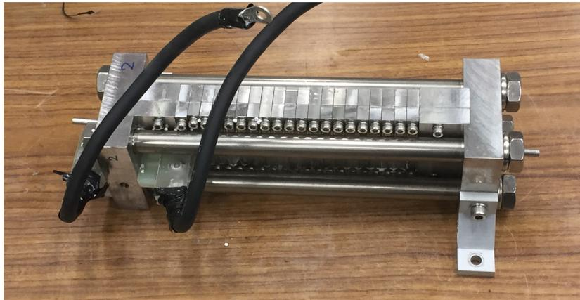
Figure 3.31: Picture of the single racetrack pulsed magnet. The total length after the reinforcement is 330 mm. A beam pipe whose diameter is 5.3 mm passed thorough the magnet.
