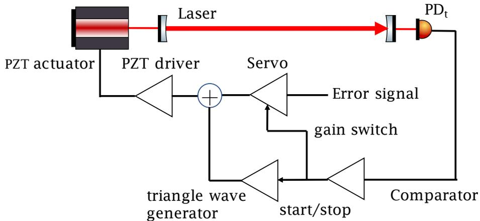
Figure 3.11: A schematic view of an auto locking system.
