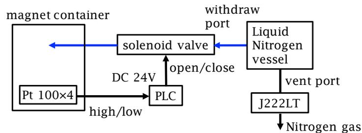
Figure 3.42: Schematic view of liquid Nitrogen serving system
