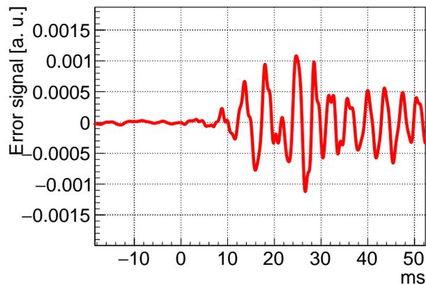
Figure 4.4: The average of the waveform of the error signal. The pulse is generated at  $t=0$ . The 200 pulsed are used for averaging. The waveform is filtered by the cavity response. From this figure, the end of the time windows is chosen to be 5 ms.
