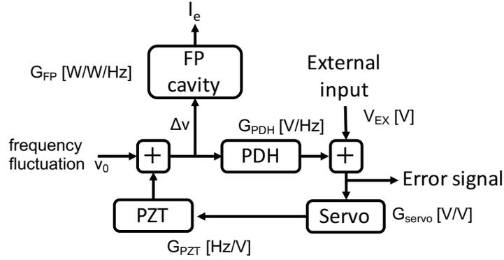
Figure 3.22: Block diagram of feedback system.
