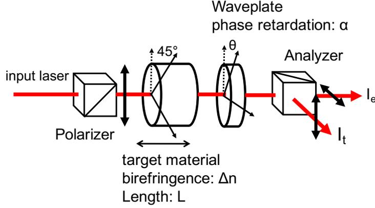
Figure 2.2: Basic setup of the polarimetry for this experiment. The target material whose birefringence is  $\Delta n$ , and length is  $L$  is placed between polarizers. A waveplate is used to induce the static birefringence. The power ratio of the output of the analyser is used to measure the ellipticity.
