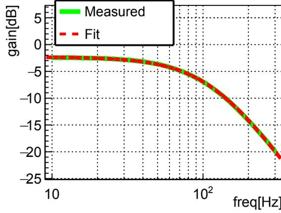
Figure 3.17: Gain curve of the transfer function from the input power modulation to the extraordinary power modulation. The measured curve with fitted by  $T_{\text{FP}}^V$ . From the fitting, the phase retardation of the Fabry-Pérot cavity is obtained
