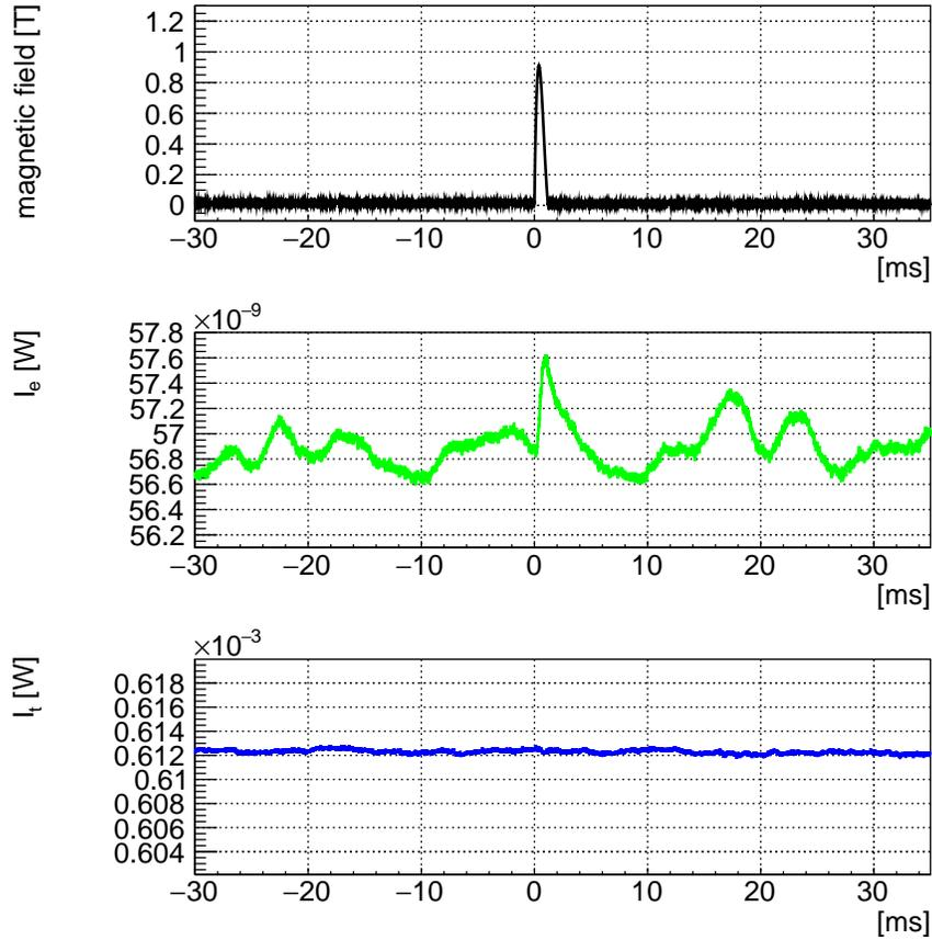
Figure 4.7: An example of the measured data of validation run. Top: magnetic field. middle:  $I_e$ . Bottom:  $I_t$ . The change of  $I_e$  after the magnetic field can be seen whereas no change can be seen in  $I_t$ . The range of the Y-axis of the middle and bottom figure is  $\pm 1.5\%$  of their DC power.
