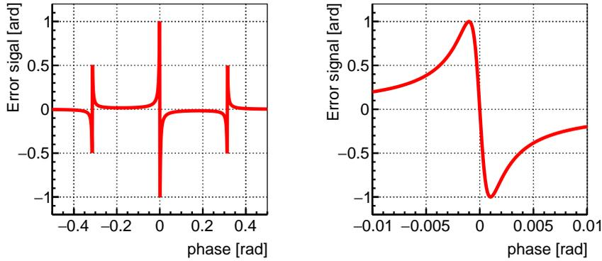
Figure A.4: Example of PDH signal as a function of a phase acquired during the trip between 2 mirrors when  $r^2 = 0.999$  and  $t^2 = 0.001$ . Left: PDH signal in wide phase region. A sharp peak can be seen around the resonance frequency. Right: PDH signal enlarged around the resonance frequency. PDH signal almost proportional to the difference between laser frequency and resonance frequency.
