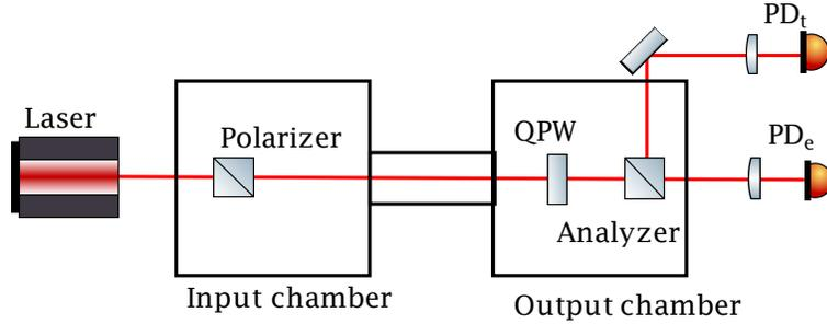
Figure 3.25: Schematic view of the set up for a birefringence measurement without a Fabry-Pérot cavity. Instead of the mirrors for a Fabry-Pérot cavity, a quarter wave plate is mounted in the output vacuum chamber. All other set up is the same with the measurement with a Fabry-Pérot cavity.
