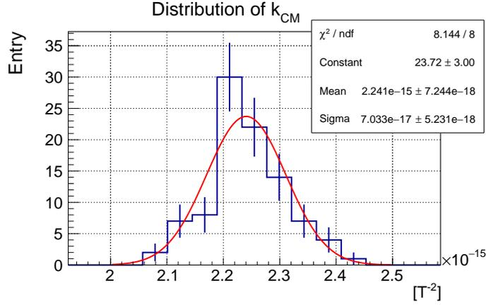
Figure 4.10: Distribution of  $k_{\text{CM}}^{\text{N}_2}$  measured at 1 kPa. The distribution is fitted by Gaussian. From the fitting result, the mean value and its error of  $k_{\text{CM}}^{\text{N}_2}$  is obtained.
