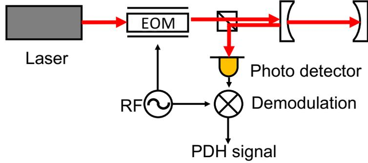
Figure A.3: Schematic of the PDH method. An EOM is used to modulate the input laser frequency. The information of the resonance frequency is implemented on the reflected light from the mirror.
