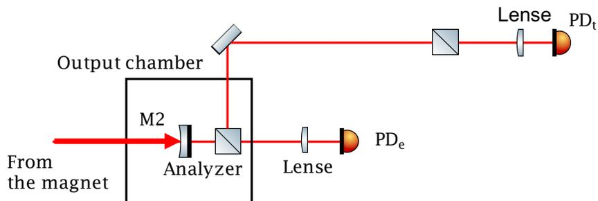
Figure 3.4: Schematic view of the output optics.
