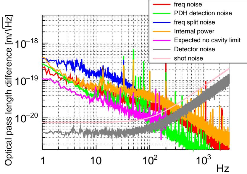
Figure 3.21: Power spectrum of the possible contribution of the all known noise source.
