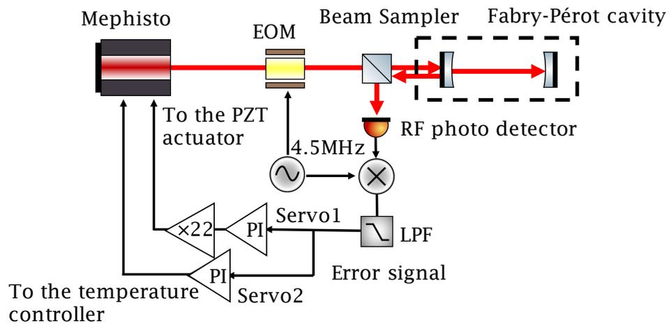
Figure 3.9: Schematic view of the frequency feedback system for a Fabry-Pérot cavity.
