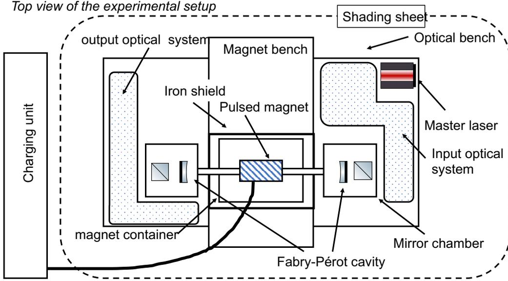
Figure 3.1: Schematic view of the experimental setup. On the  $1.2 \text{ m} \times 2.4 \text{ m}$  optical bench, optical system is installed. A Pulsed magnet are installed on the magnet bench. The magnet is connected to the charging unit via coaxial cable outside the laser booth.
