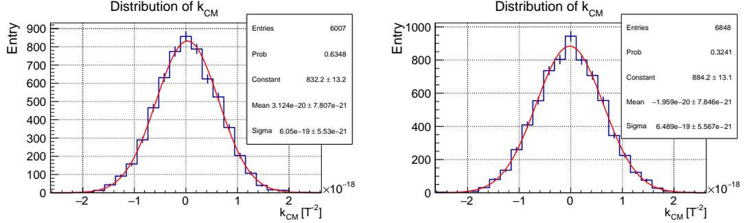
Figure 4.21: Distribution of  $k_{CM}$  assuming the noise on  $I_t$  appears on  $I_t$  only. Left:  $k_{CM}$  obtained during B-1 and B-2. Right:  $k_{CM}$  obtained during C-1 and C-2. Each distribution is fitted by Gaussian. From the fitting result, the mean value and its error of  $k_{CM}$  is obtained.
