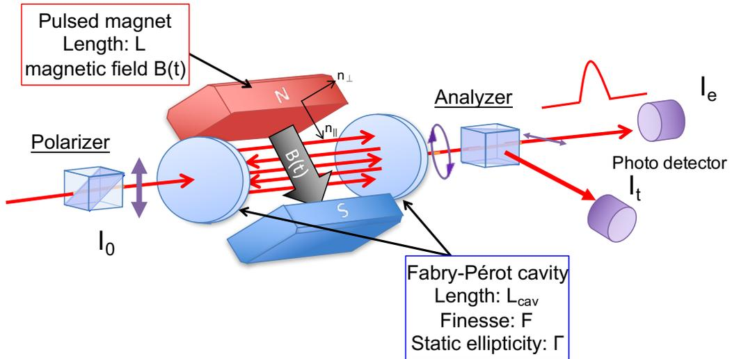
Figure 2.1: Overview of the experimental setup to measure VMB. A strong pulsed magnet is used to induce large  $\Delta n$ . A Fabry-Pérot cavity is used to enhance the effective interaction length and to induce the static birefringence. From the output power of the analyzer, the ellipticity is measured.
