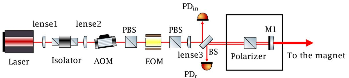
Figure 3.3: Schematic view of the input optics.
