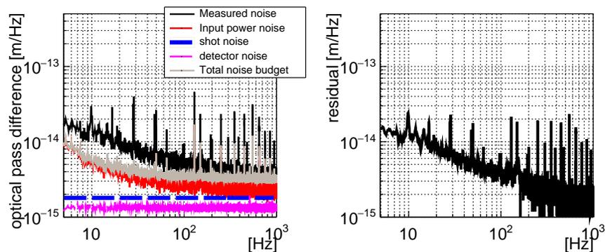
Figure 3.26: Left: noise spectrum of the optical pass difference without a Fabry-Pérot cavity. Black line: measured noise. Gray line: Estimated total noise budget from all known noise source. Right: The residual between measured noise and estimated noise budget.
