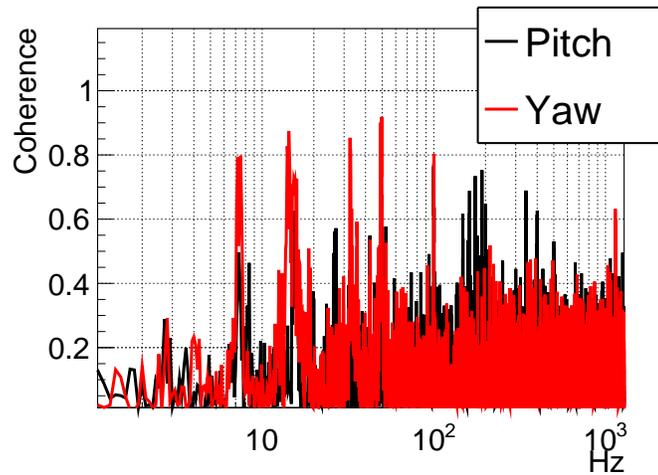
Figure D.3: The coherence spectrum of the birefringence noise spectrum and pointing noise of the reflected light. No strong coherence can be observed except for some sharp peaks.
