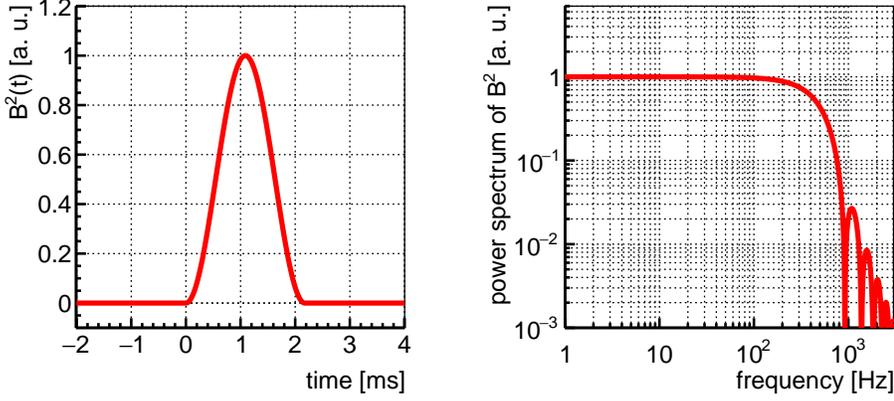
Figure 2.5: Example of square of the magnetic field with pulsed magnet. Assumed parameter is  $C = 6$  mF and  $L = 80$   $\mu$ H. Left: Signal shape in time domain. Right: Signal spectrum in frequency domain.
