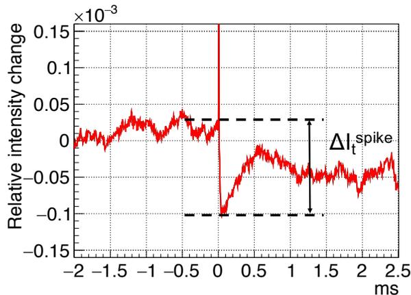
Figure 4.17: Example of the noise on  $I_t$ . The waveform is average of the 50 cycle of  $I_t$  (100 shots) after the cancellation of the effect proportional to the magnetic field. At  $t = 0$ , the magnetic field is generated. The sudden change of the output intensity ( $\sim 0.01\%$ ) is observed at the same time with the beginning of the magnetic field.
