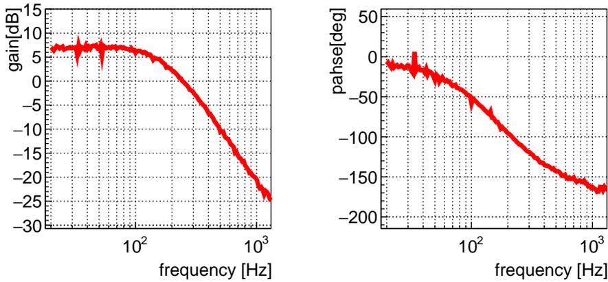
Figure 3.23: Example of the measured transfer function from  $V_{\text{ext}}$  [V] to  $V_e$  [V]. This function is used to estimate the contribution of frequency noise to the optical pass length noise spectrum.
