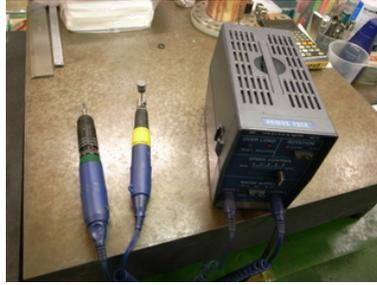
Figure 5.14: The Leutor with a carbide blade and a grind stone.
