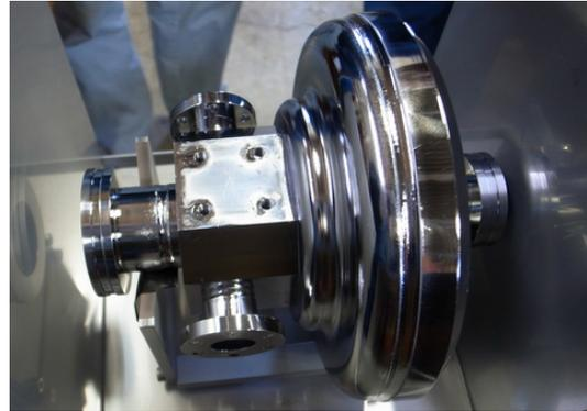
Figure 5.23: The manufactured two-mode cavity after the annealing.
