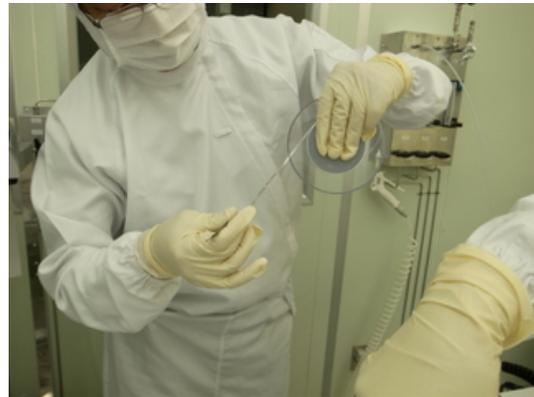
Figure 5.25: The indium ribbon for the sealing.
