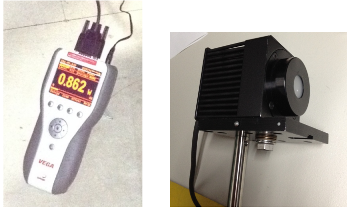
Figure 5.9: ( left) The power meter (VEGA, Ophir Photonics) used for measuring total laser power. ( right) The sensor attached to the power meter.
