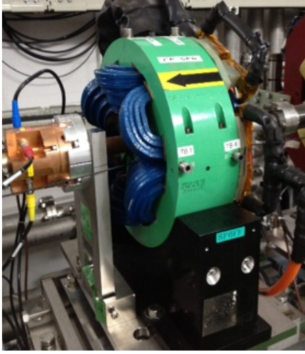
Figure 1.8: (top) the Final Doublet quadrupole magnets at ATF2, QF1 (yellow) and QD0 (red), shown together with the FFS sextupole magnets interleaved with the FD. (bottom left) A close-up view of the SD0, the sextupole magnet placed next to the QD0. (bottom right) One of the skew setpoles in the FFS for correction of nonlinear errors.
