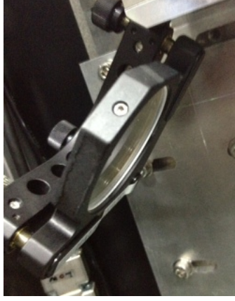
Figure 3.15: (left) The half mirror on the vertical table which split the laser beam into upper and lower paths which cross at the IP to form the interference fringes against which the e^- beam collides.
