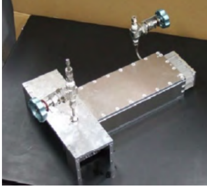
Figure 3.26: The structure of the Shintake Monitor gamma-ray detector. [25]
