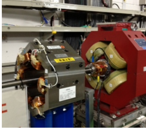
Figure 1.8: (top) the Final Doublet quadrupole magnets at ATF2, QF1 (yellow) and QD0 (red), shown together with the FFS sextupole magnets interleaved with the FD. (bottom left) A close-up view of the SD0, the sextupole magnet placed next to the QD0. (bottom right) One of the skew setpoles in the FFS for correction of nonlinear errors.
