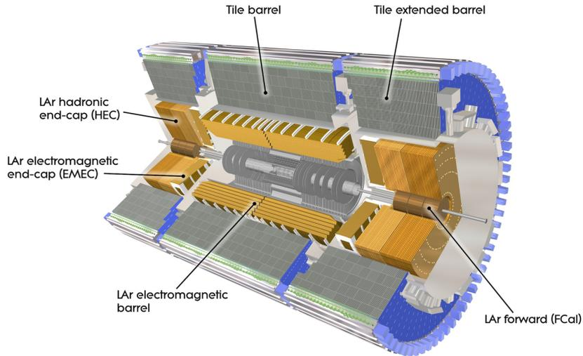
Figure 13: Schematic overview of ATLAS Calorimeter system.
