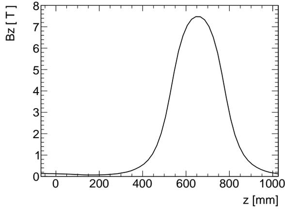
Figure A.4: Simulated magnetic field  $B_z$  on the  $z$ -axis (by CST PARTICLE STUDIO). The emitter ring is at  $z=0$  mm, and the RF cavity is at 650 mm.
