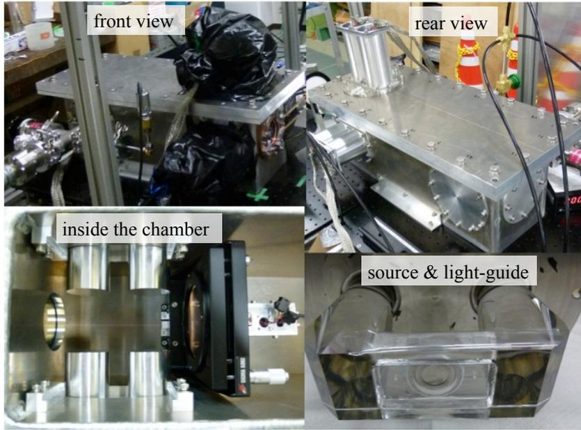
Figure 2.28: Photograph of the chamber.
