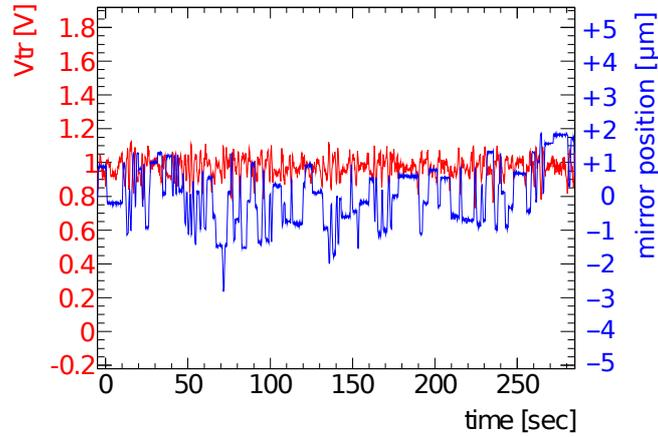
Figure 2.27: Accumulated power stabilized by control of the mirror position.
