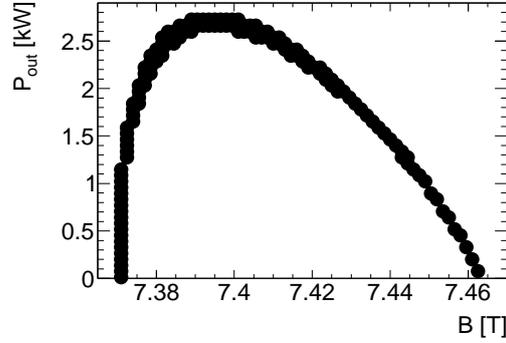
Figure A.7: Calculated output power of the gyrotron. Operation parameters are cathode voltage  $V_k = -18$  kV, beam current  $I_b = 500$  mA, magnetic field  $B = 7.4$  T, cavity radius  $R_2 = 2.475$  mm, beam radius  $R_b = 0.7 \cdot R_2$ , and pitch factor  $\alpha = 1.2$ .
