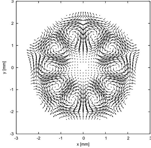
Figure A.2: Transverse structure of the electric field in the RF cavity (TE<sub>52</sub> mode).
