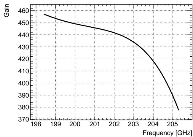
Figure 2.15: Expected Gain of the Fabry-Pérot cavity in case of plane wave input.
