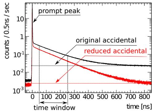
Figure 3.7: Time spectrum obtained by time difference of the  $\text{LaBr}_3(\text{Ce})$  signal and plastic scintillator one. Time window for delayed coincidence is shown as a region between two black dashed lines. The black and red solid lines show before and after accidental rejection, respectively.
