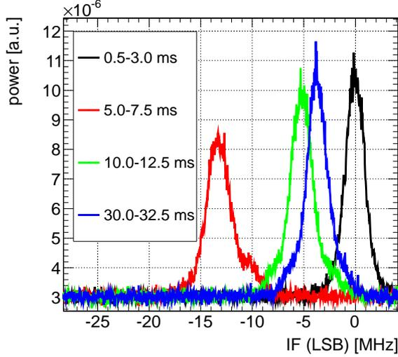
Figure 2.6: Measured frequency spectra of FU CW G1. IF of LSB is shown. Different lines correspond to different delay time from the rising edge of pulse. A time range for FFT is 2.5 ms. One spectrum is a result of the average of 100 cycles.
