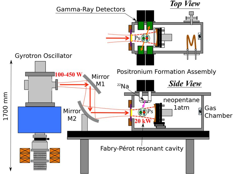
Figure 2.1: Schematic view of our experimental setup.
