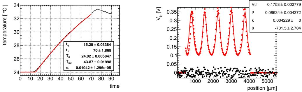
Figure 2.23: Data fitting for the power calibration. (left) Measurement of  $P_{\text{in}}$  with the temperature increase of water. Black points are measured data, and a red line is the best fit. (right) Measurement of  $V_{\text{tr}}$  by moving the piezoelectric stage near the mesh mirror position. Black points are data when the chopper is closed, and red points are measured data. A red line is the best fit.
