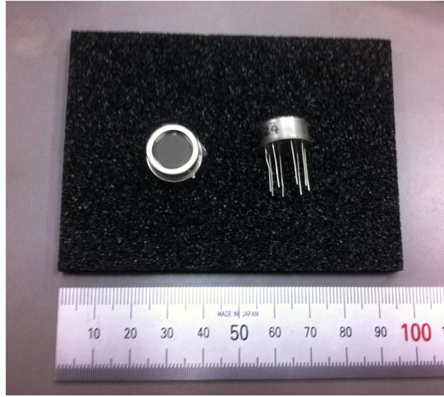
Figure 2.18: Pyroelectric detectors (Spectrum Detector Inc. SPH-49).
