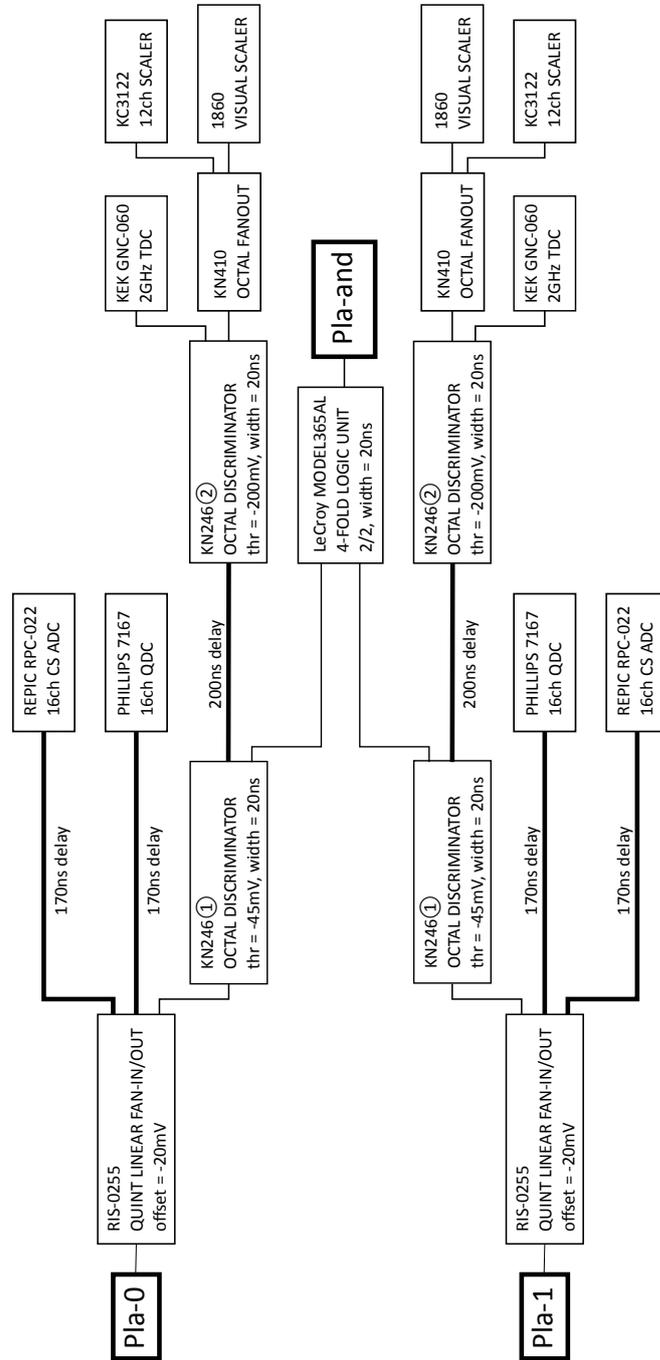
Figure 2.37: Circuit diagram for plastic scintillator system.
