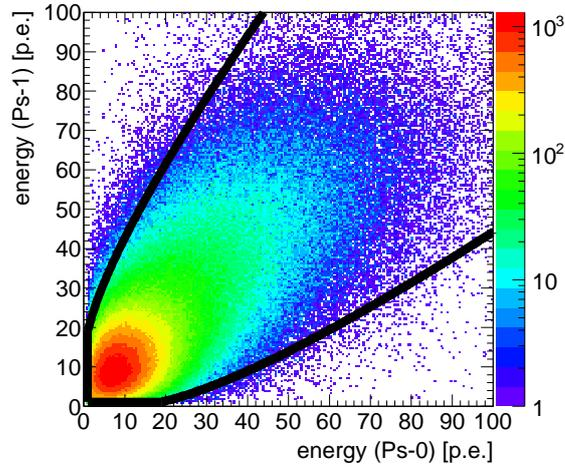
Figure 3.5: 2D energy spectrum of plastic scintillator. The region inside black lines is selected.
