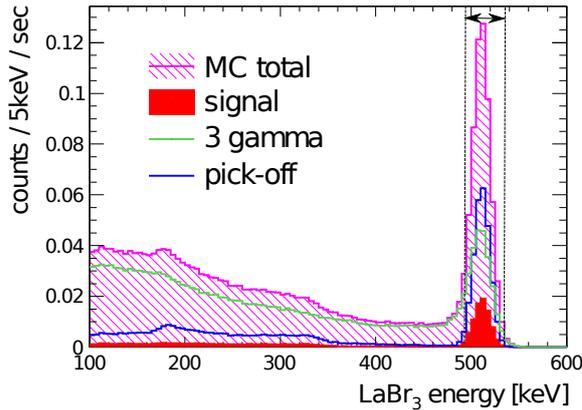
Figure 3.9: Expected energy spectrum of LaBr<sub>3</sub> (Ce) scintillators with Monte Carlo simulation.  $f = 203.4$  GHz and  $P_{\text{acc}} = 20$  kW. 511 keV is required at the opposite side of the back-to-back pairs.
