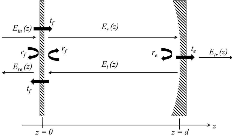
Figure 2.11: Schematic view of a Fabry-Pérot resonant cavity.
