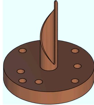
Figure A.11: Schematic view of the helical launcher.
