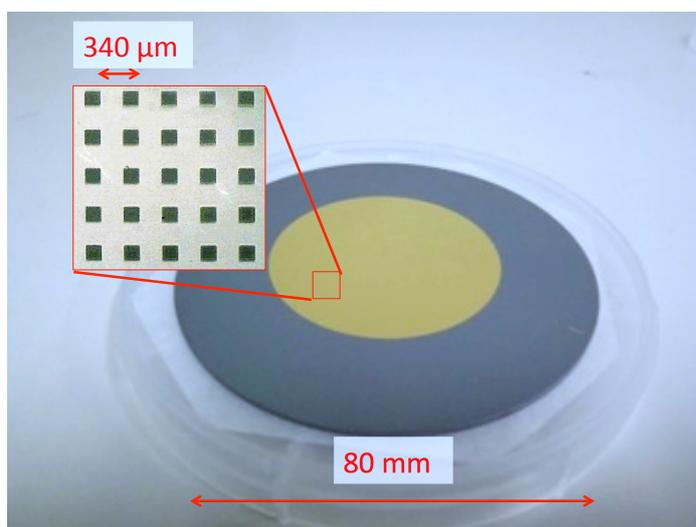
Figure 2.16: Photograph of gold mesh on silicon substrate.
