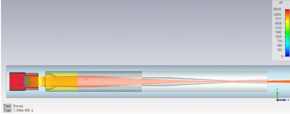
Figure A.5: Simulated electron trajectories from the MIG (by CST PARTICLE STUDIO).
