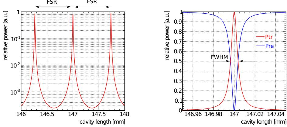
Figure 2.12: Calculated resonances of the Fabry-Pérot resonant cavity. The left shows neighboring resonances. The right represents comparison of  $P_{tr}/P_{in}$  (red line) and  $P_{re}/P_{in}$  (blue line).  $\lambda$  is 1.47 mm,  $\mathcal{F}$  is 100, and  $\beta$  is 1 (critical coupling).
