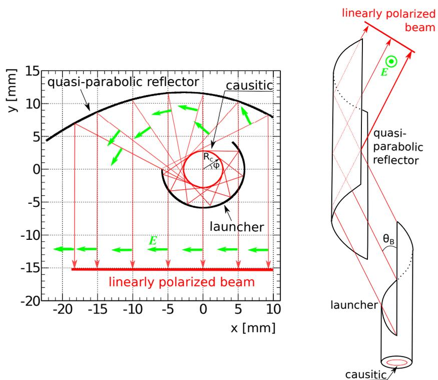
Figure A.12: Schematic view of Gaussian converter. (left) Top view. (right) Side view.
