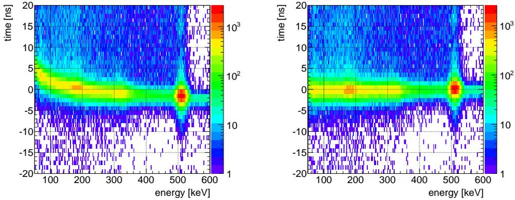
Figure 3.3: 2D plots of time vs energy deposited in one LaBr<sub>3</sub>(Ce) scintillator. (left) Before the time-walk correction. (right) After the correction.
