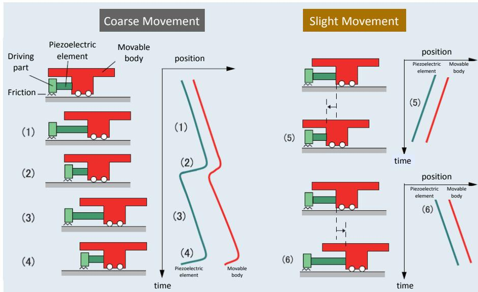
Figure 2.17: Principle of operation of an SIDM<sup>TM</sup> (Smooth Impact Drive Mechanism) actuator.
