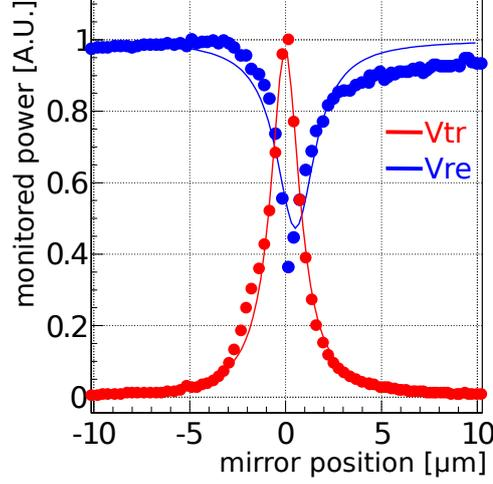
Figure 2.20: Measured resonance of the Fabry-Pérot cavity arrangement. The red points are voltage of transmitted power  $V_{tr}$ , and the blue points are that of reflected power  $V_{re}$ . The solid lines are the best fitting results of each data. The peak position is adjusted to the origin of the horizontal axis. Input frequency is 203.7 GHz.
