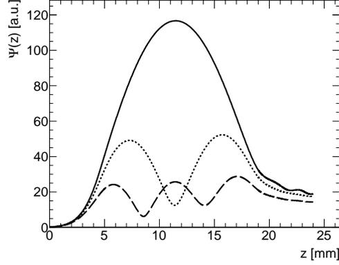
Figure A.3: Axial structure of the electric field in the RF cavity. Solid, dots, and dashed lines show  $\text{TE}_{521}$ ,  $\text{TE}_{522}$ ,  $\text{TE}_{523}$ , respectively.
