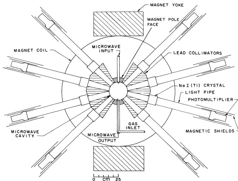
Figure 1.7: Schematic view of the previous experiment [31].
