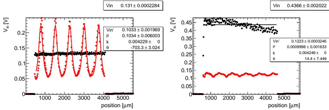
Figure 2.24: Data fitting for the reflection correction. Black points are data in phase of  $P_{in}$  measurement (no reflection), and red points are data in that of  $V_{tr}$  measurement. Solid lines are the best fits for each data. The end point mirror moves a few wavelength near the mesh mirror position of the Fabry-Pérot cavity. (left) Small correction case. (right) Large correction case.
