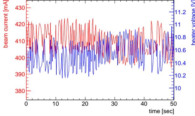
Figure 2.26: Electron beam current stabilized by heater-voltage feedback.
