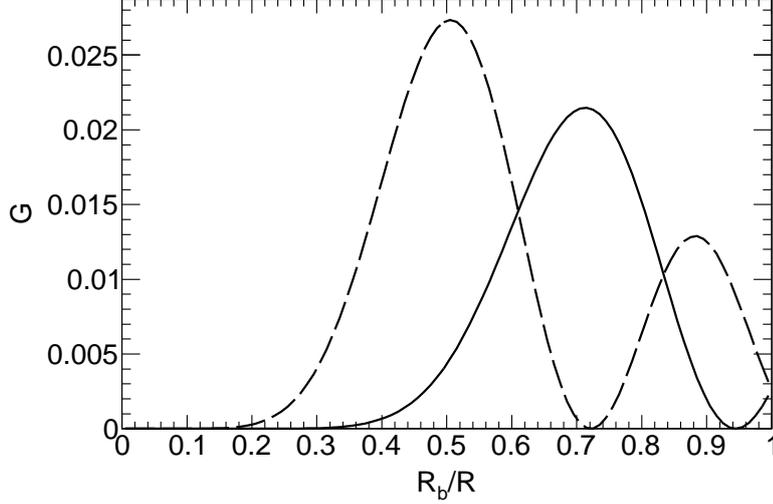
Figure A.6: Coupling factor of the  $TE_{52}$  mode. Solid line shows the counter-rotating mode, dashed one shows the co-rotating mode.
