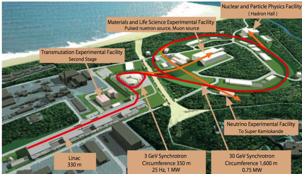
**Figure 3.3:** A bird's view of the J-PARC accelerator [43].
