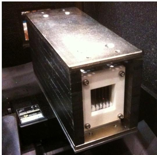
**Figure 3.10:** A photograph of a magnetic supper mirror (MSM).
