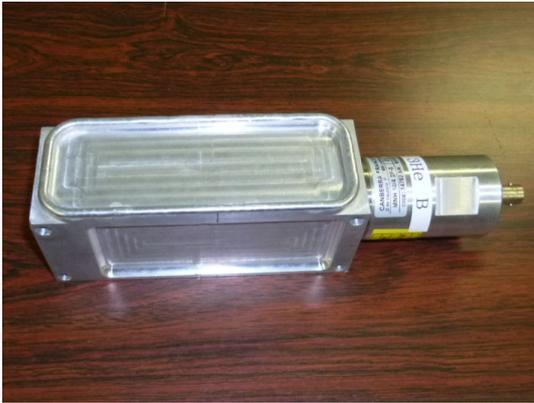
**Figure 3.19:** A photograph of a beam monitor.
