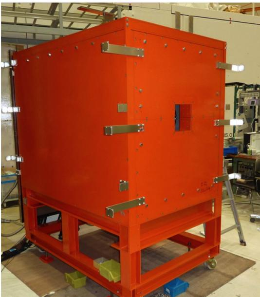
**Figure 3.23:** A photograph of the Pb shielding.
