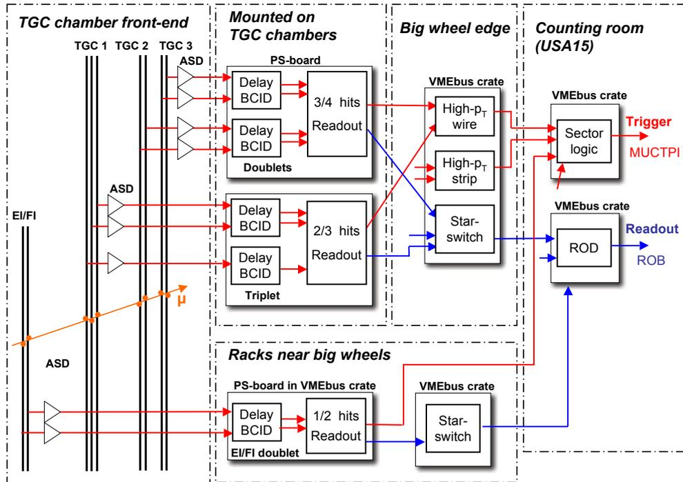
**Figure 5.10:** A schematic view of the TGC electronics system.
