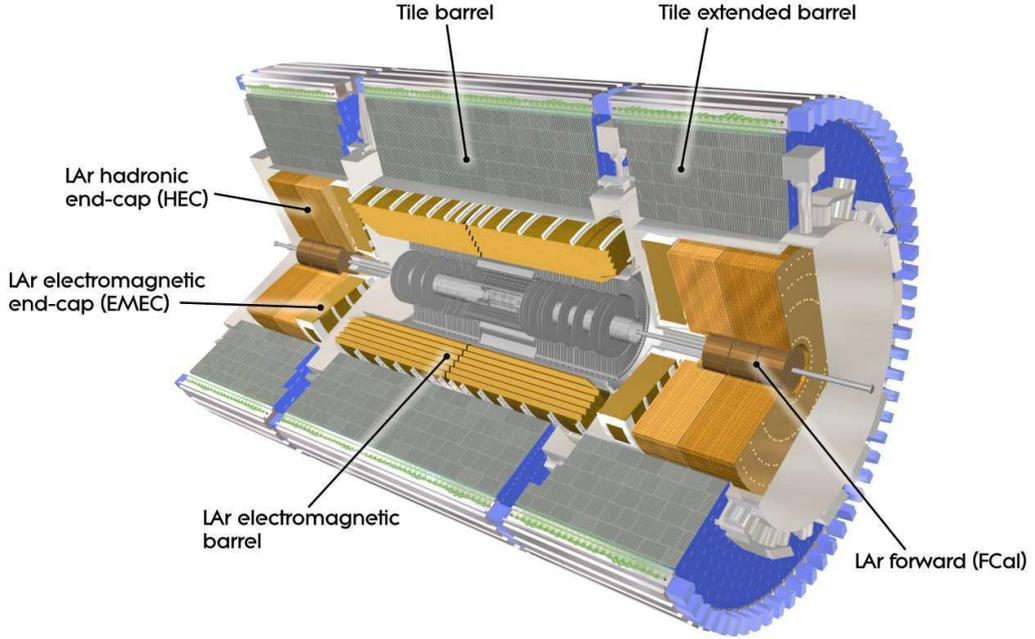
**Figure 4.11:** A cutaway view of the ATLAS Calorimeters.
