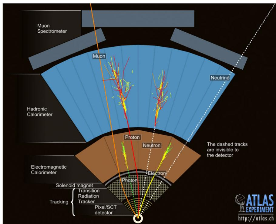
**Figure 4.2:** Particle detection in the ATLAS detector.
