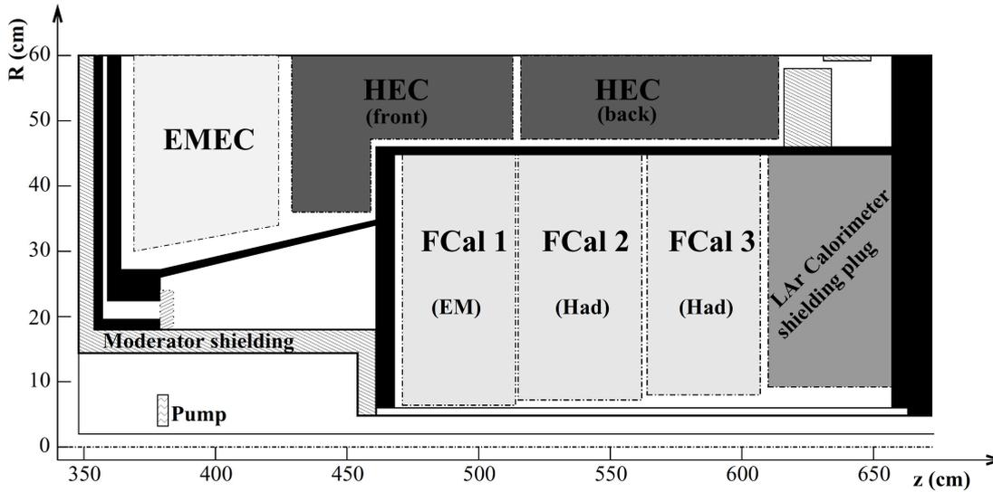
**Figure 4.18:** The layout of the calorimeters in the endcap and forward region. All the calorimeters are housed in the same cryostat.
