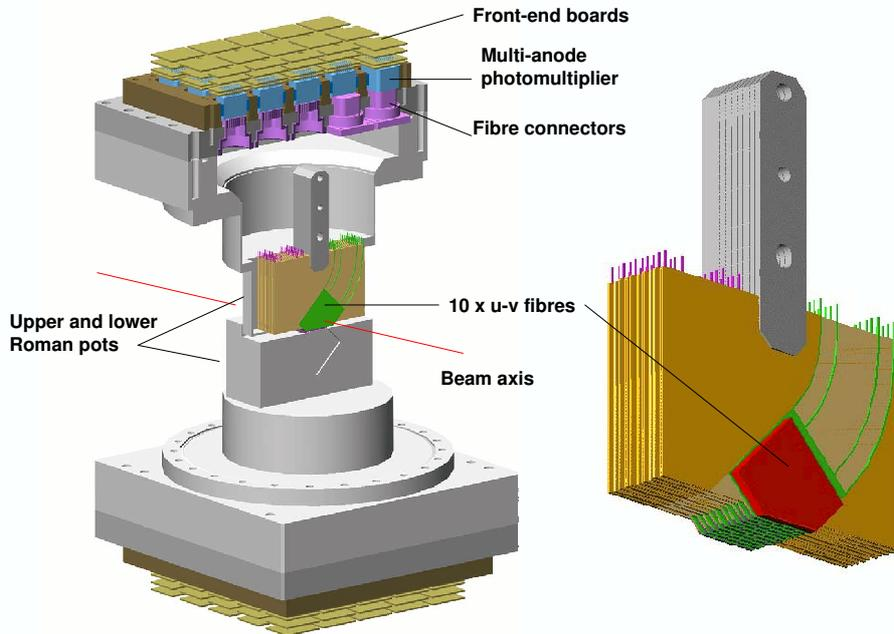
**Figure 4.34:** A schematic view of the ALFA detector in the Roman Pot.
