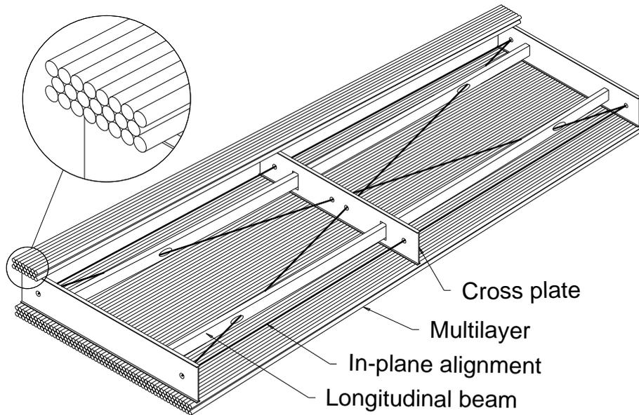
**Figure 4.26:** A schematic view of a barrel MDT chamber.
