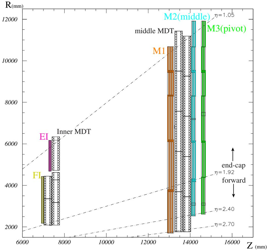
**Figure 5.7:** The cross section in  $R - Z$  plane of the TGC system.
