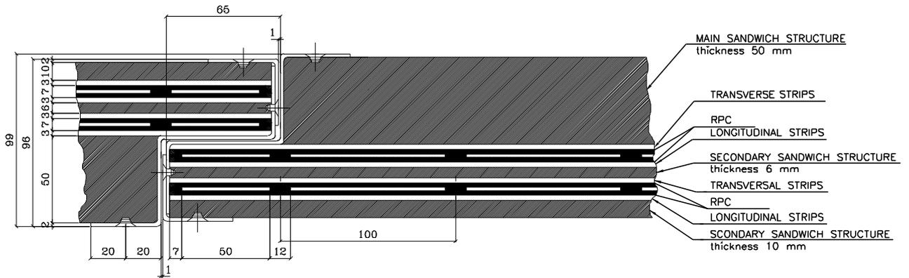
**Figure 4.32:** The cross section of a RPC chamber.
