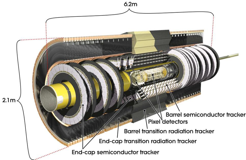
**Figure 4.5:** A cutaway view of the ATLAS Inner detector (ID).
