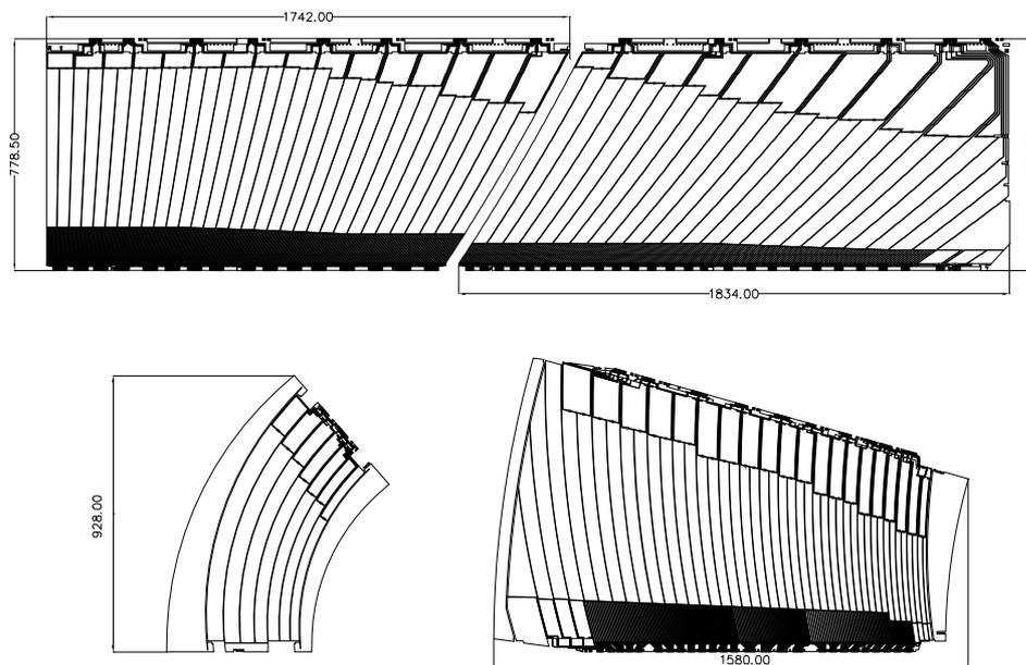
Figure 4.15: The layout of the signal layers in the EM calorimeters in  $r - z$  plane. The figures on top are for the barrel and the extended endcap. The figure on bottom-left is for the endcap inner and bottom-right is for the endcap outer wheels.
