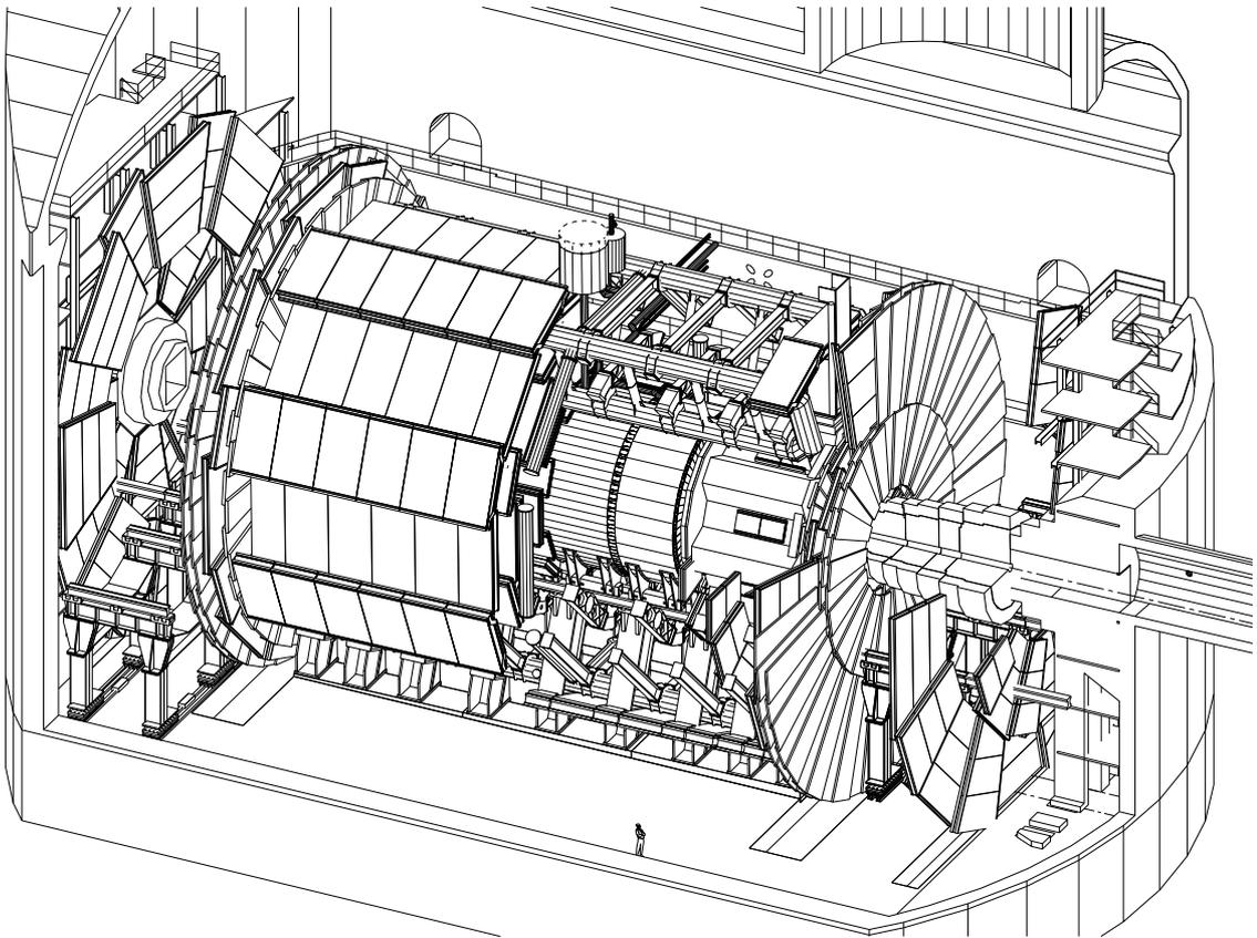
**Figure 4.24:** 3-D view of the ATLAS detector in the underground hall. The muon chambers (partly removed to show the inner structures) are arranged in three layers around the inner detector and the calorimeter in the space between 5 and 10 m in radius and 7 and 23 m distance from the interaction point.
