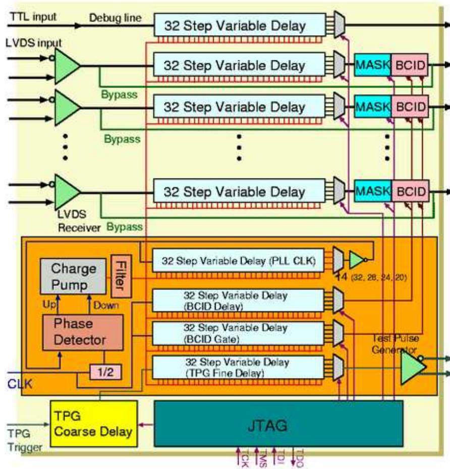
Figure 5.11: A block diagram of the Patch-Panel.
