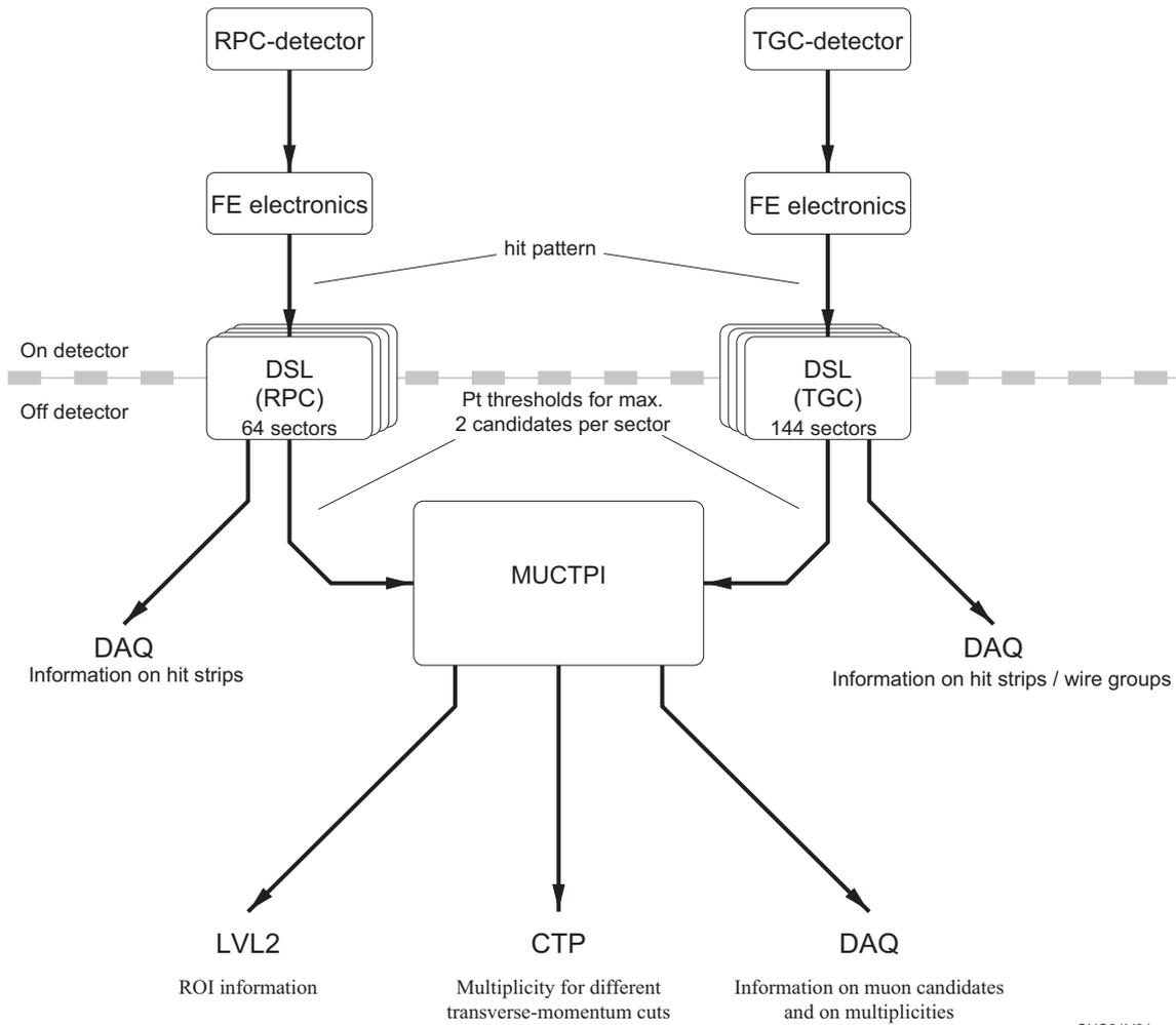
**Figure 5.6:** A schematic drawing of the ATLAS L1 muon trigger.
