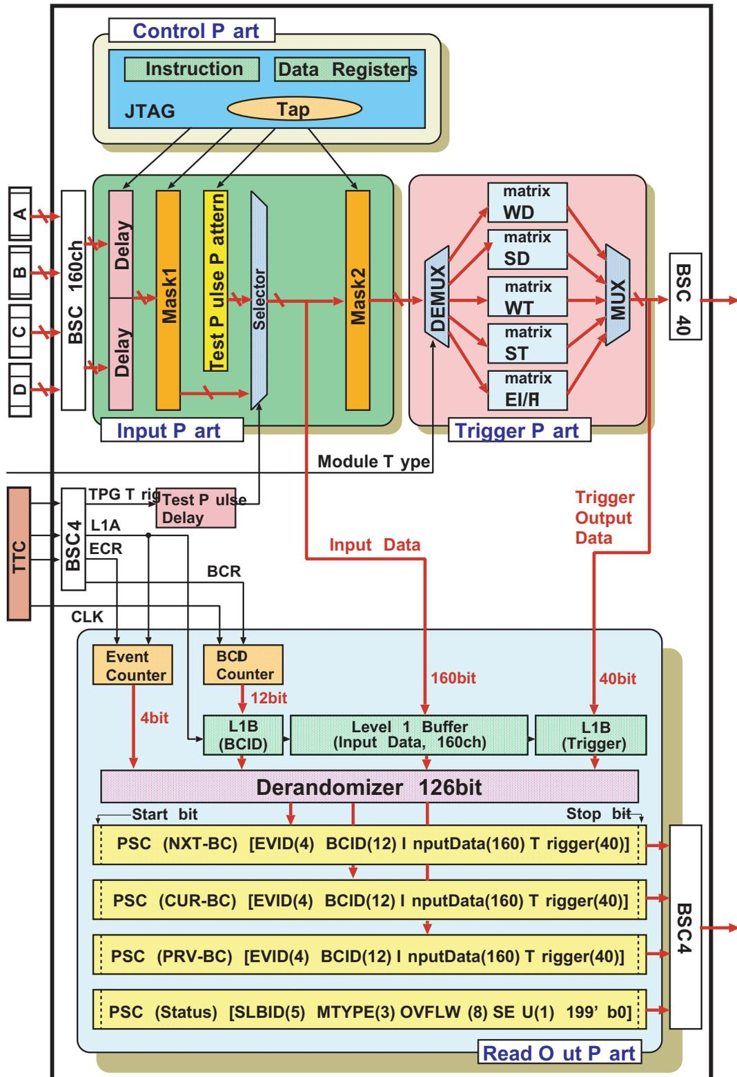
Figure 5.14: A block diagram in the SLB ASIC.
