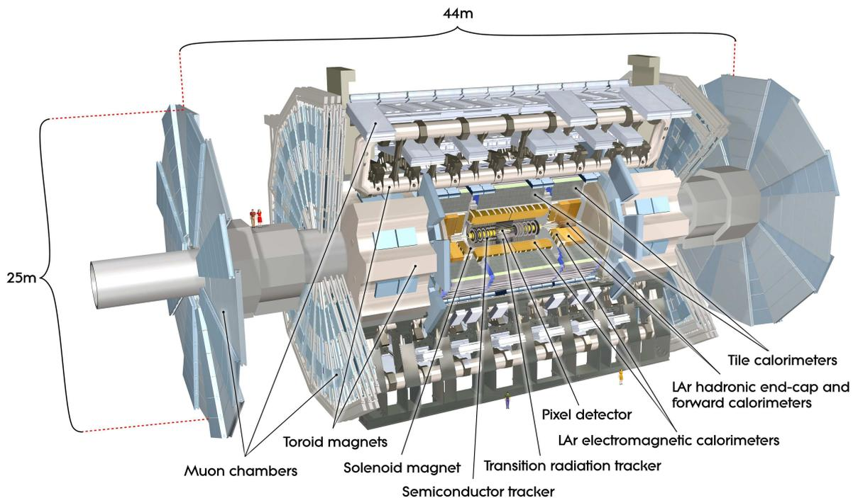
**Figure 4.1:** A cutaway view of the ATLAS detector.
