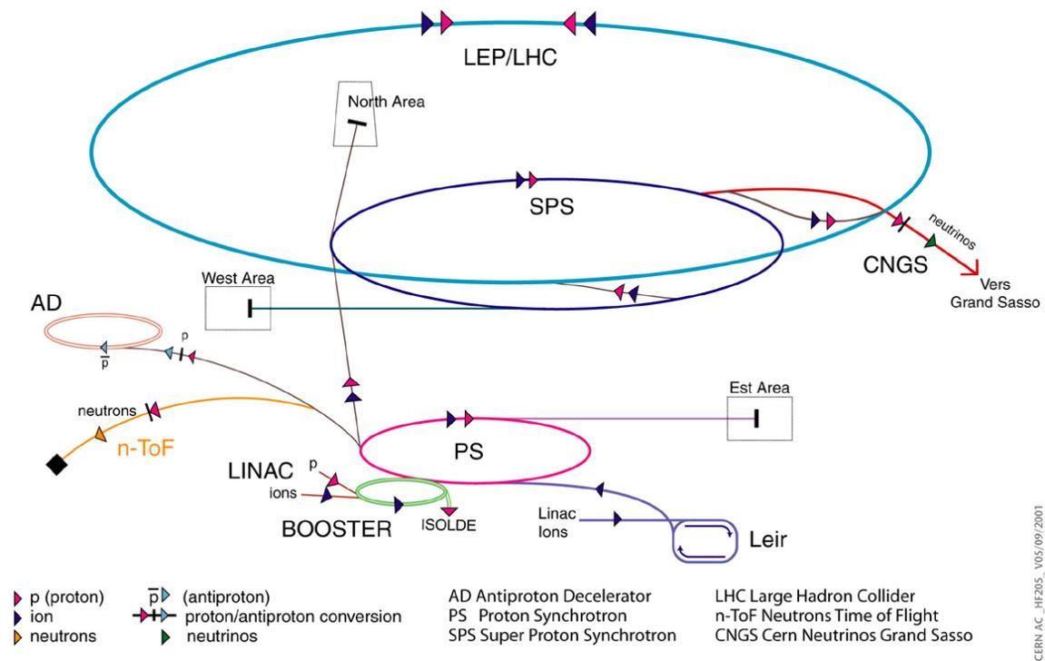
**Figure 3.1:** A schematic view of the LHC complex
