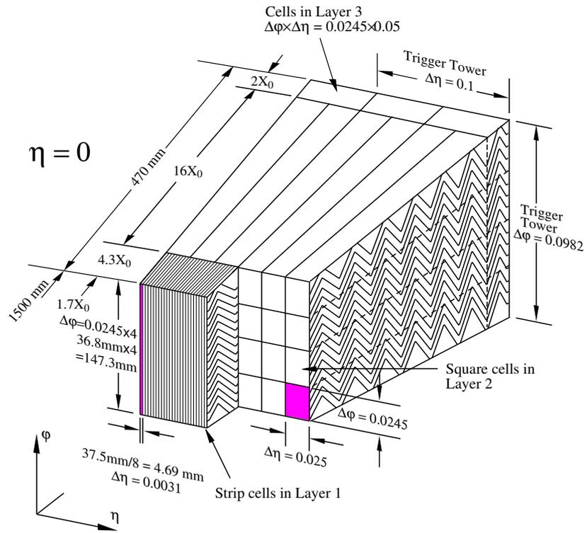
Figure 4.14: Sketch of a barrel LAr Calorimeter module.
