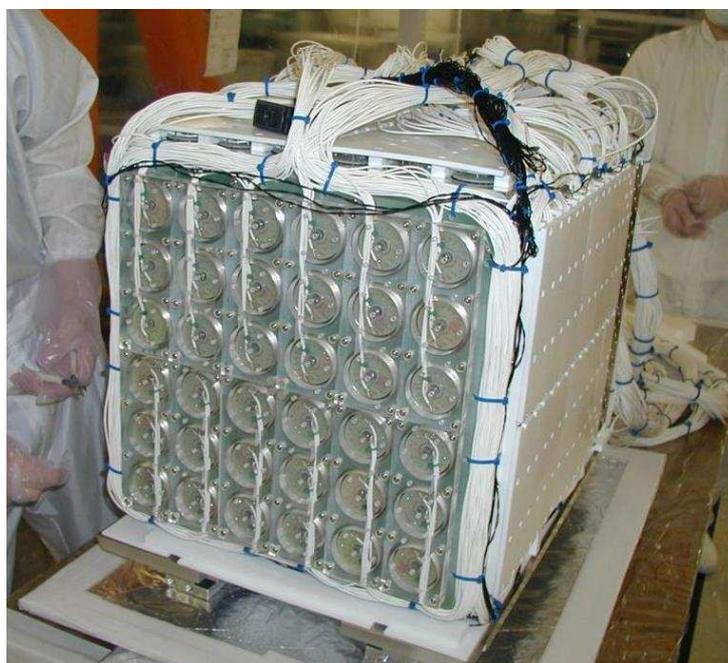
Figure 3.6: (a) Schematic view of the PMT holder. (b) Picture of the PMT holder in the 100-liter prototype detector from the front. Front face structure is mainly made of G10 and acrylic.
