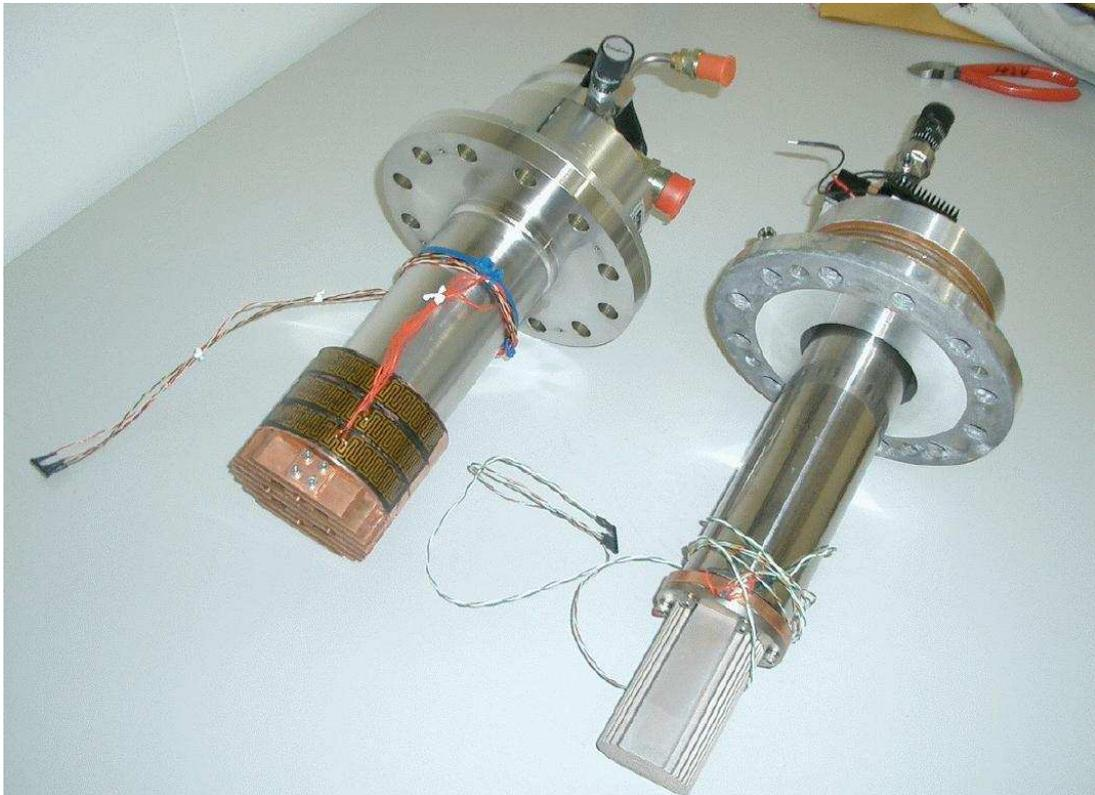
Figure 3.10: Pulse tube used in the refrigerator of the LXe detector. The right is the pulse tube for the 100-liter prototype with a cooling power of 70 W at 165 K. The left is the latest version which will be used in the final detector and its cooling power is improved up to 190 W at 165 K.
