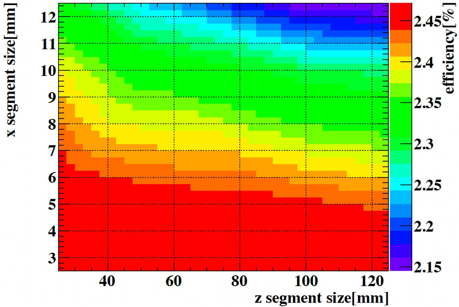
efficiency in 3 mm thickness LYSO
