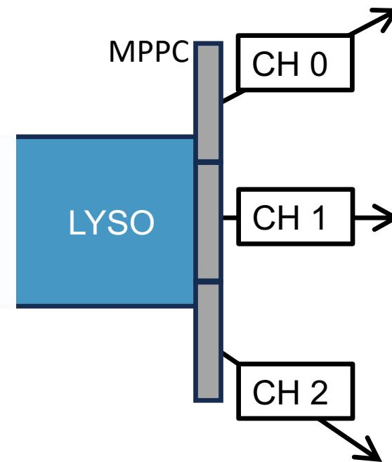
center MPPC channels (larger p.e.) are weighted more than the edge MPPC channels (smaller p.e.)
