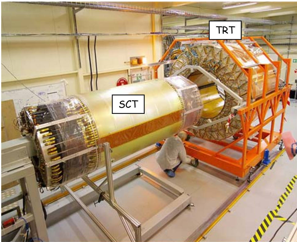
In February, barrel Si detector (SCT) was inserted into barrel TRT. → Installation in the pit in Aug. 2006
