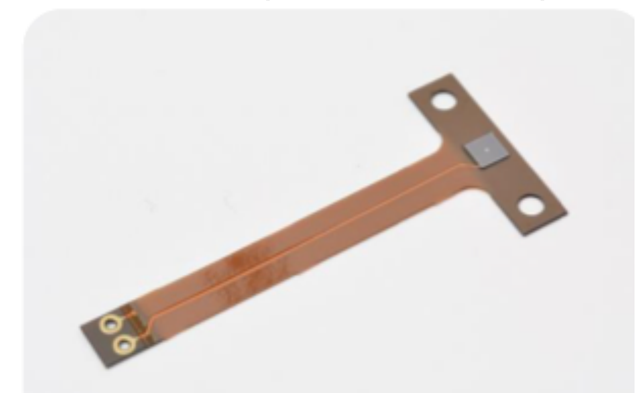
VUV-MPPC chip on film (CoF) package
