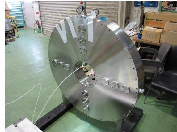
Pressuring with nitrogen gas
