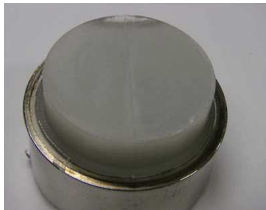
Figure 3.7: A filler is attached to the rear of PMT using the mold
