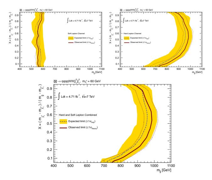
Figure C.9: Exclusion limits at 95% CL with the simplified model gluino pair production with  $X = (m_{\tilde{g}} - m_{\tilde{\chi}_1^{\pm}})/(m_{\tilde{g}} - m_{\text{LSP}})$  samples fixing the LSP mass at 60 GeV for the soft lepton channel (top-left), hard lepton channel (top-right) and combined results (bottom), respectively.
