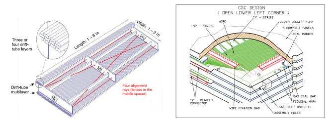
Figure 3.14: Structure of MDT (left) and CSC (right)
