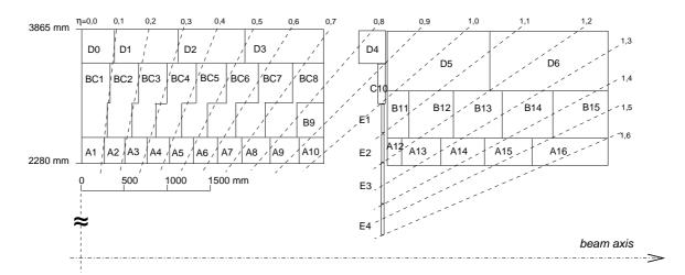
Figure 3.12: Segmentation of tile calorimeter modules in center (left) and extended barrels (right)
