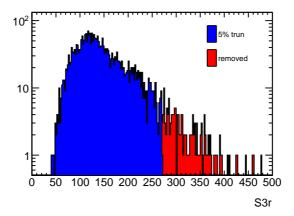
Figure D.4: Distribution of the energy deposition in the S3 in ADC channel units. The higher energy deposition events rejected by applying 5% truncation. The remaining events (MIP-like events) and the rejected ones are in blue and red, respectively.
