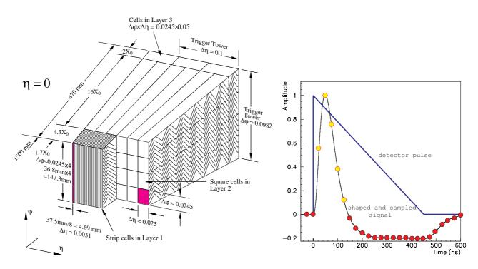
Figure 3.9: A sketch of LAr barrel module (left) and the raw and converted signal shape of LAr (right).
