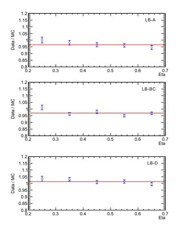
Figure D.9: The distribution of ratios between the data and the MC samples and fitting results obtained applying the Maximum Likelihood Method for the LB-A, LB=BC and LB-D layers , respectively. The beam energy is equal to 20 GeV.
