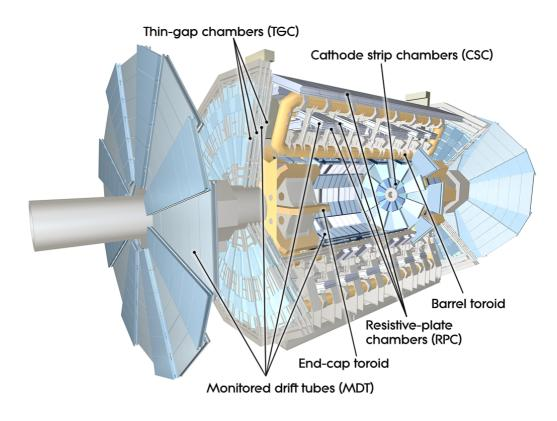
Figure 3.13: Cut-away view of ATLAS muon system
