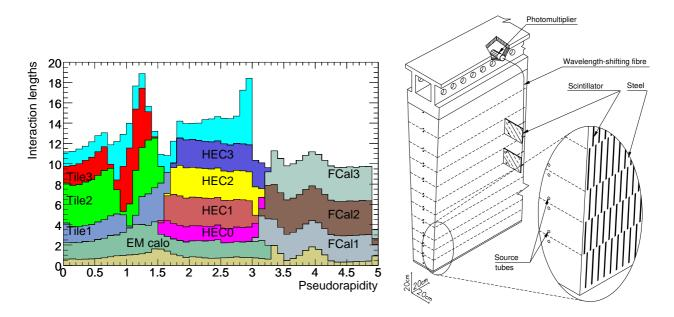
Figure 3.11: Left : Cumulative amount of material in unit of interaction length  $\lambda_0$  for electromagnetic calorimeter, hadronic calorimeter and total amount of material in front of the first active layer of the Muon spectrometer ( $|\eta| < 3.0$ ). Right : Schematic of module of tile calorimeter
