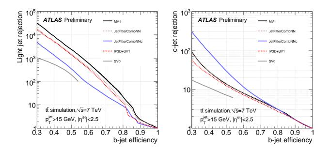
Figure B.12: Light flavour jet rejection (left) and c-hadron jet rejection as a function of the b-tag efficiency for the each b-tag algorithm based on  $t\bar{t}$  MC samples.
