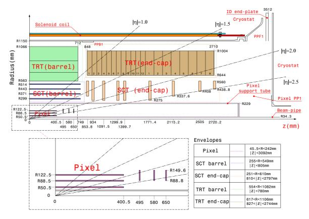
Figure 3.6: Plane view of a quarter-section of the ATLAS inner detector showing each of the major detector elements with its active dimensions and envelops.
