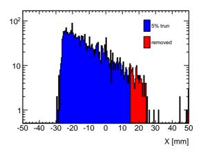
Figure D.5: Distribution of the x-coordinate of the impact point of the muon in the BC2 chamber. The events far from beam core are rejected by applying 5% truncation. The remaining events (beam core events) and rejected events are in blue and red, respectively.
