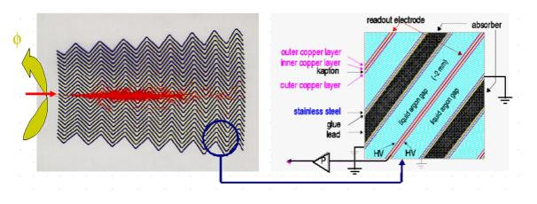
Figure 3.8: Shower shape in LAr calorimeter and fine structure of it.
