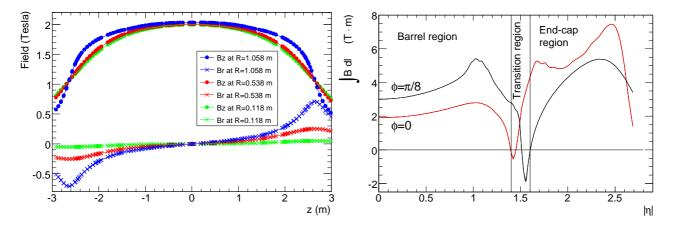
Figure 3.5: (Left) : Magnetic field components in the inner cavity along r- and z-dependence of the radial (Br) and axial (Bz) at fixed azimuth. The lines are fitting results. (Right) : Predicted integral magnetic field as a function of  $|\eta|$  from the innermost to the outermost MDT layer in one toroid octant for infinite momentum muons. The curves correspond to azimuthal angles  $\phi = 0$  (red) and  $\phi = \pi/8$  (black).
