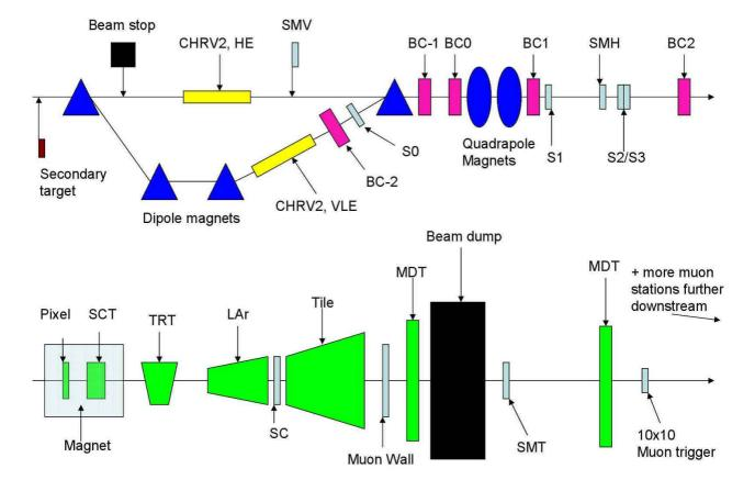
Figure D.3: Schematic outline of the beam line instrumentation, and also of the ATLAS sub-detector elements. In this test beam, the scintillators (S1, S2, S3) and beam chambers (BC0, BC1, BC2) were installed. The beam energy were determined by bending at dipole magnets. The muons fired the muon trigger.
