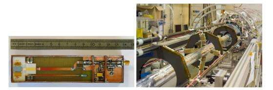
Figure 3.18: Top view of a BCM module in left picture, showing the diamond sensors (left side of picture), HV supply and signal-transmission lines, two amplification stages and signal connector (right side of picture). Close-up view one BCM station in right picture installed at 184 cm from the center of the pixel detector, which can be seen at the far end of the picture.
