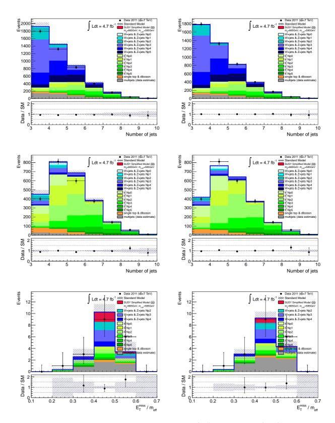
Figure C.6: Simultaneous fit results in HistFitter before fitting (left) and after fitting (right). Used signal model is simplified SUSY model at  $m_{\tilde{g}} = 665$  GeV,  $m_{\text{LSP}} = 585$  GeV.
