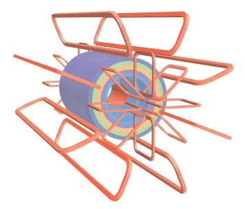
Figure 3.4: Structure of eight barrel and end-cap toroid coils and four solenoid layers.
