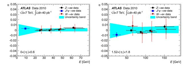
Figure B.1: Correction factors of the electron energy scale as a function of  $E_{\rm T}$  in  $Z \to ee$  and  $J/\psi \to ee$  events.
