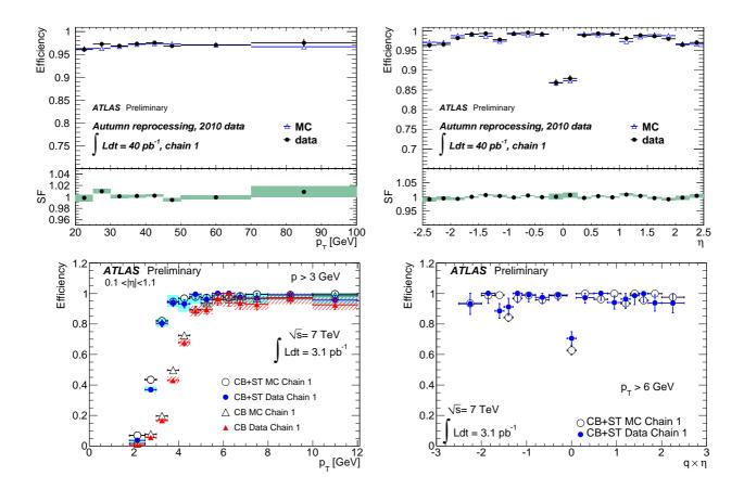
Figure B.6: Efficiencies and correction scale factor of the muon as a function of  $p_{\rm T}$  (top-left) and  $\eta$  (top-right) for the high  $p_{\rm T}$  muon and efficiencies of the low  $p_{\rm T}$  muon as a function of  $p_{\rm T}$  (bottom-left) and  $\eta$  (bottom-right) in  $Z \to \mu\mu$  and  $J/\psi \to \mu\mu$  events.
