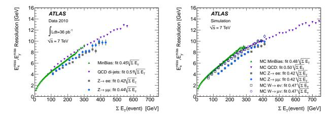
Figure B.18:  $E_{\rm T}^{\rm miss}$  resolution of both observed data (left) and MC simulation (right) as a function of the total transverse energy in the event calculated by summing the  $p_{\rm T}$  of muons and the total transverse energy in the calorimeter. The resolution of the two  $E_{\rm T}^{\rm miss}$  components is fitted with a function of  $\sigma = k\sqrt{\Sigma E_{\rm T}}$  and the fitted values of the parameter k, expressed in GeV<sup>1/2</sup>. [70]
