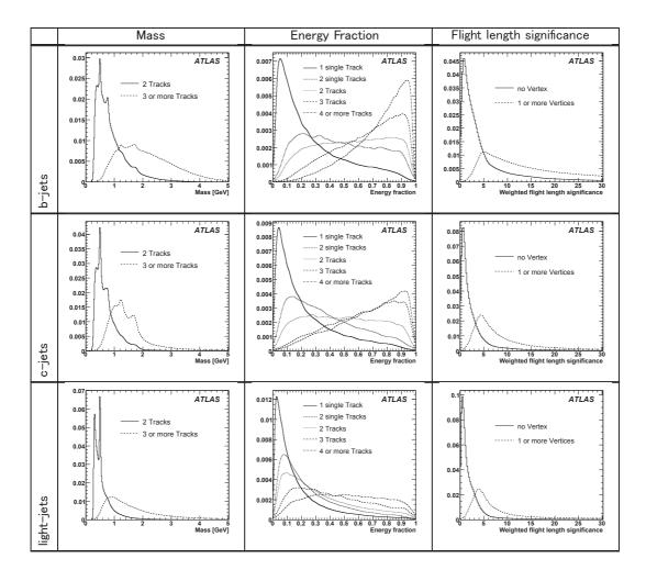
Figure B.13: Probability density function (PDF) of the parameters to identify the b-jet, c-jet and light flavor jet.
