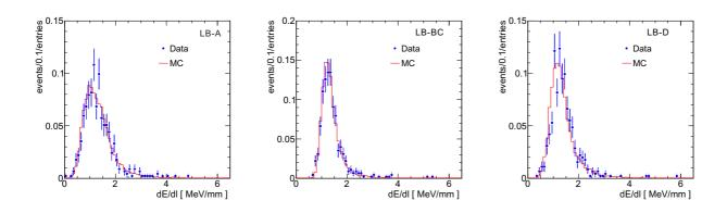
Figure D.6: The distribution of  $dE/d\ell$  obtained in the LB-A, LB-BC, and LB-D layers using muons with energy equal to 20 GeV and  $\eta$  equal to 0.25. The data and MC events are shown by filled circles and solid lines, respectively. The distributions are normalized to one.
