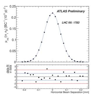
Figure B.20: Specific interaction rate versus nominal beam separation for the EventOR algorithm of BCM (horizon) in the x plain at May 15th 2011. The residual deviation of the data from the Gaussian plus constant term fit, assuming statistical error only, is shown in the bottom panel.
