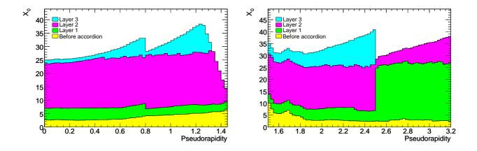
Figure 3.10: The cumulative amount of material in the unit of radiation length  $X_0$  for the electromagnetic calorimeter in the barrel region (left) and end-cap region (right).
