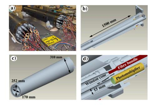
Figure 3.19: (a) Picture of the two LUCID vessels fully assembled and ready to be installed in ATLAS; (b) Sketch of LUCID integrated in the cone supporting the beam pipe; (c) Design of the gas vessel; (d) Expanded view of the readout area showing the coupling between the 15 mm diameter Cherenkov tubes and the photomultiplier tubes.
