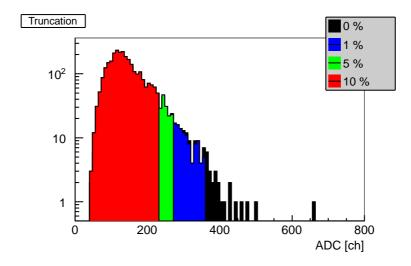
Figure D.10: Distribution of energy deposition in S3 and the region separated by the truncation at 10%, 5%, and 1%, respectively.
