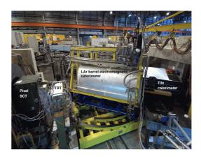
Figure D.1: Schematic view of the test beam table setup.
