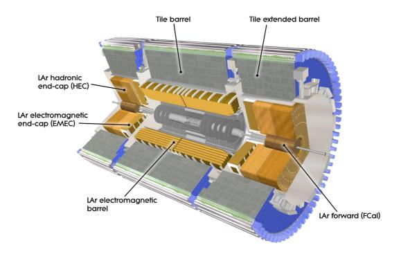
Figure 3.7: The cat-away view of the calorimeter system
