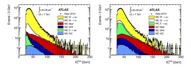
Figure B.16:  $E_{\rm T}^{\rm miss}$  distributions both data and MC predications with the  $W \to e\nu$  events (left) and  $W \to \mu\nu$  events (right). The MC samples are normalized by entries of data and the theoretical cross section. [70]
