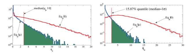
Figure C.2: Distributions both  $f(\tilde{q}_{\mu}|\mu=0)$  and  $f(\tilde{q}_{\mu}|\mu=1)$  and relation to the median $[q_{\mu}|\mu=0]$  (left) and median $[q_{\mu}|\mu=0]$ -1 $\sigma$  (right) [71]. The  $\pm 1, \pm 2\sigma$  band of the expected limit estimated these distributions.
