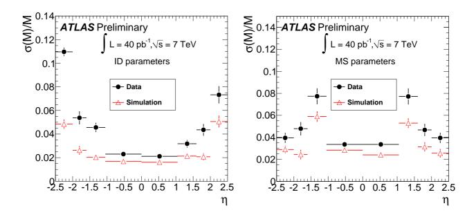
Figure B.5: The muon momentum resolution as a function of  $\eta$  for the inner detector (left) and muon spectrometer (right).
