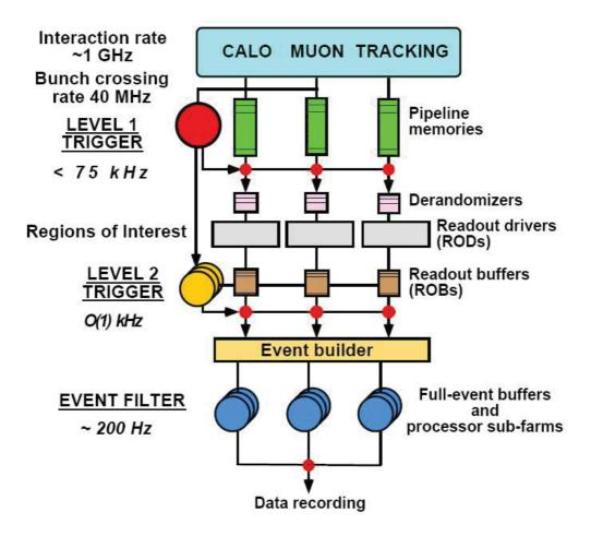
Figure 3.16: ATLAS Trigger system
