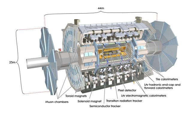
Figure 3.3: Cut-away view of ATLAS detector. Dimensions of the detector are 25 m in height and 44 m in length. Overall weight of the detector is approximately 7000 tones.
