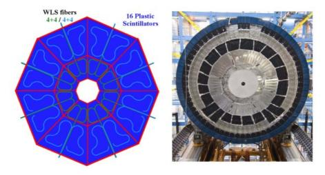
Figure 3.17: Schematic (left) and photo (right) of MBTS.
