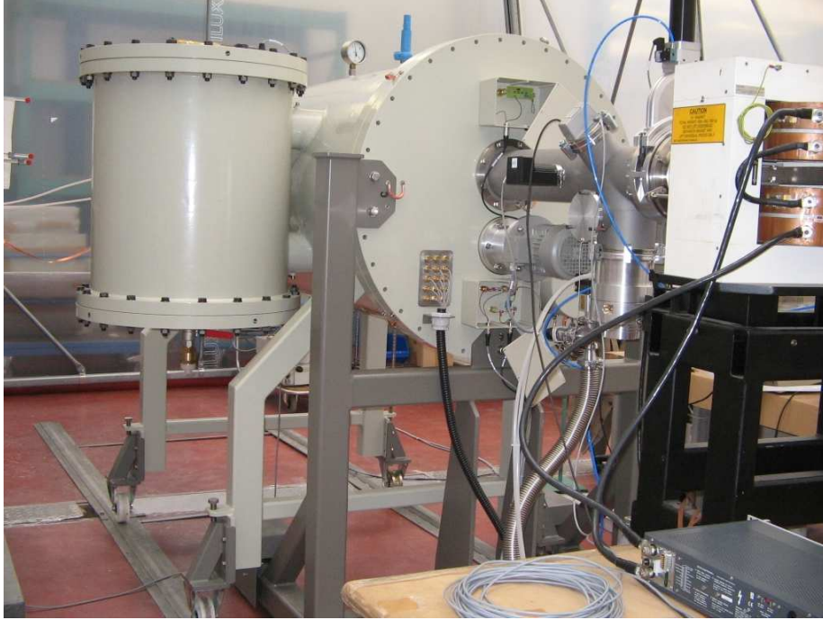
Figure 2.17: C.W. accelerator seen from the front. RF coil is on the left.
