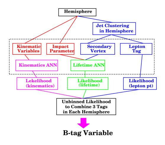
Figure 4.17: The scheme of b-tagging algorithm, LB.
