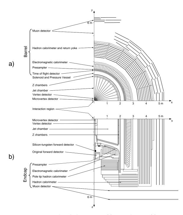
Figure 3.4: The quarter of the OPAL detector in (a) the the front and (b) top views.
