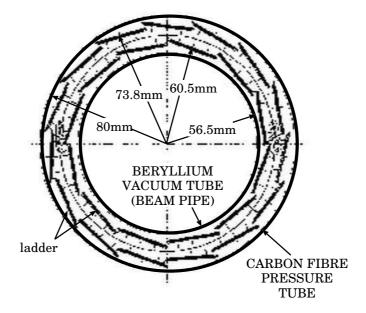
Figure 3.5: Silicon Microvertex Detector
