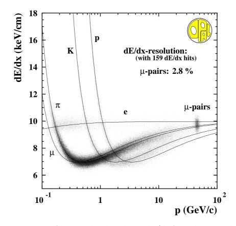
Figure 3.7: Distribution of measured and predicted dE/dx for hadronic tracks and muon pairs as a function of the momentum (p). The dE/dx resolution for the muon-pairs with 159 hits used for the dE/dx calculation was 2.8%.
