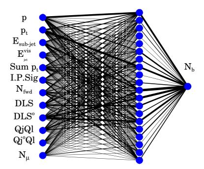
Figure D.4: An example of the constructed ANN ( $\mathcal{N}_{b}$  for muon). The width of the line indicated the strength of the coupling for the two nodes.
