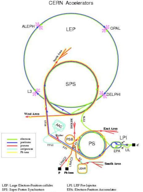
SPS: Super Proton Synchrotion AAC: Anti proton Accumulator Complex ISOLDE: Isotope Separator OnLine DEvice PSB: Proton Synchrotron Booster PS: Proton Synchrotron EPI: Electron-Positron Accumulator EPA: Electron-Positron Accumulator LIL: LEP Injector LINAC LINAC: LINear Accelerator LEAR: Low Energy Antiproton Ring
