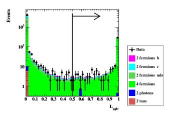
Figure 4.9: The W<sup>+</sup>W<sup>-</sup>  $\rightarrow q\bar{q}\ell\bar{\nu}_{\ell}$  likelihood discriminant  $(\mathcal{L}_{q\bar{q}}\ell\bar{\nu}_{\ell})$  distribution. The arrow indicates the W<sup>+</sup>W<sup>-</sup>-selection cut of  $\mathcal{L}_{q\bar{q}}\ell\bar{\nu}_{\ell} > 0.5$ .
