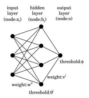
Figure D.1: The structure of the feedforward multilayer parceptron with one hidden layer.
