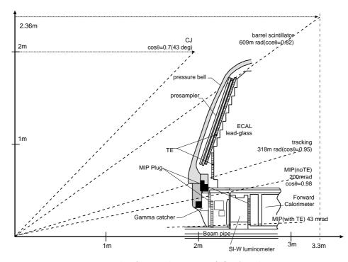
Figure 3.8: The forward region of OPAL detector.
