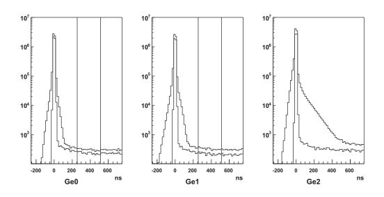
Figure 3.16: Time spectra of Ge detectors without silica target. The inside histogram is the spectrum after the SRT cut. The long tail of the spectrum after the SRT cut comes from the o-Ps in the air. The slow rise-time component of the prompt peak spreads over 200 ns for Ge0 (Ge1) and 600 ns for Ge2. The vertical lines show the region used for the evaluation of the  $3\gamma$  SRT efficiency.
