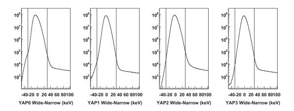
Figure 3.10: Narrow-Wide spectra for YAP scintillators The events within  $\pm 30$  keV are selected. The two vertical lines shows the boundaries of the cut.
