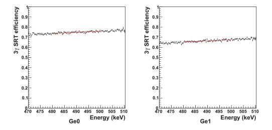
Figure 3.18:  $3\gamma$  SRT cut efficiency of Ge detectors. The event ratio before and after the SRT cut is plotted along the energy. The spectrum is fitted with linear function from 480 keV to 500 keV and the function is used as the  $3\gamma$  SRT cut efficiency. Ge0:  $1.023(150) \times 10^{-3} E(\text{keV}) + 0.247(73)$ , Ge1:  $1.063(153) \times 10^{-3} E(\text{keV}) + 0.143(75)$
