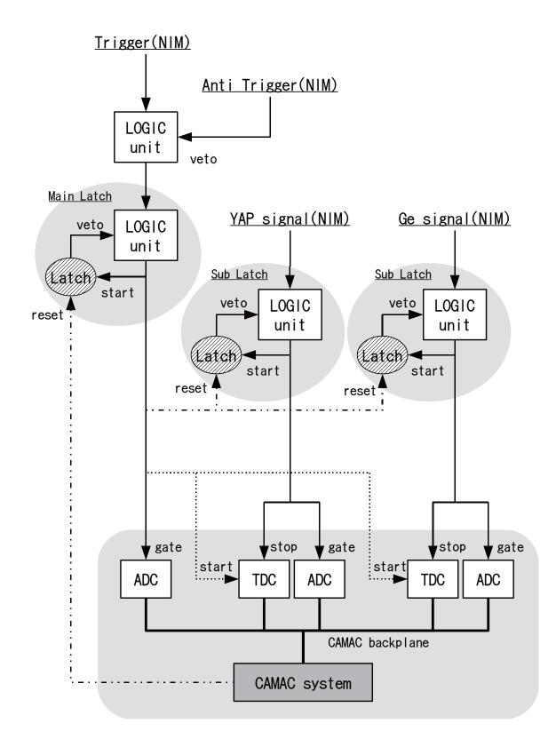
Figure 2.10: Schematic diagram of the process data-flow.
