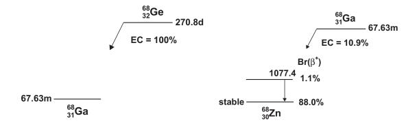
Figure 2.4: The level diagram of the <sup>68</sup>Ge isotope. The <sup>68</sup>Ge nucleus decays to the <sup>68</sup>Ga nucleus through the electron capture (left diagram). Then, the <sup>68</sup>Ga nucleus decays to the <sup>68</sup>Zn nucleus through the  $\beta^+$  decay (right diagram).
