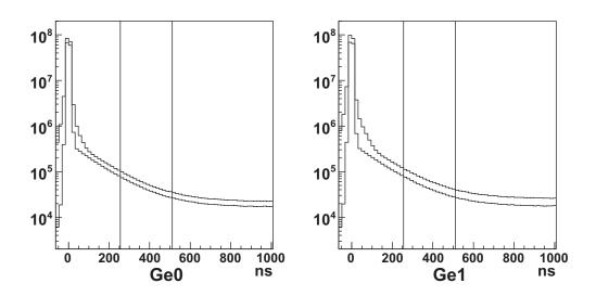
Figure 3.17: Time spectra of Ge detectors. The inside histogram is the spectrum after the SRT cut. The time region within the two vertical lines is used for the evaluation of the  $3\gamma$  SRT efficiency.
