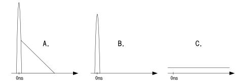
Figure B.2: Time distribution of the the  $\gamma$ -rays. The  $\gamma$ -rays which hit the detectors in this experiment are classified into three groups. **A.** Ps events, **B.** source related events, **C.** accidental events.
