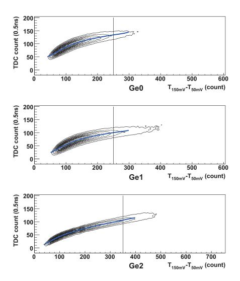
Figure 3.14: Time walk of Ge detectors. The detection time of the prompt peak is plotted against the rise-time variable  $(T_{150 \ mV}-T_{50 \ mV})$ . The prompt peaks for every 20 counts regions of the rise-time variable is fitted with seven order polynomial function. The blue line shows the fitted polynomial function and the time walk is corrected by this function. The slow rise-time component beyond the vertical line is eliminated.
