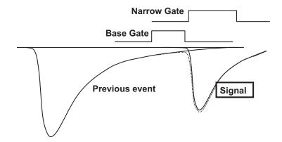
Figure 3.4: The schematic of the Base cut. The Base cut rejects the events where the preceding signal disturbs the timing and the energy information of the succeeding signal.
