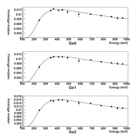
Figure 2.7: The relative peak efficiency of the germanium detectors. Measured data using the <sup>152</sup>Eu source are plotted with closed circles as a function of  $\gamma$ -ray energy. The continuous line represent the relative efficiencies estimated with the Monte Carlo simulation. The data is normalized so as to fit the simulation.
