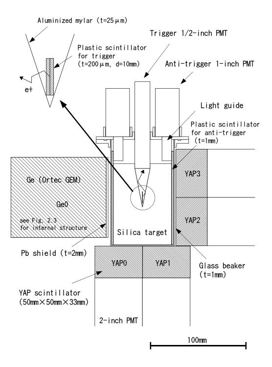
Figure 2.2: Schematic diagram of apparatus (side view).
