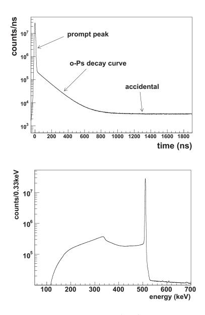
Figure 3.2: Time and Energy spectrum of the Ge detector. The upper figure is the time spectrum of the Ge detector. The energy range is restricted from 300 keV to 520 keV and the time walk correction is already applied. The lower figure is the energy spectrum of the Ge detector. The time window is restricted before 700 ns. The lower energy region is suppressed by the slow rise-time cut.
