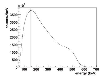
Figure 3.27: Energy spectrum of YAP scintillator in the delayed region. The time region is restricted from 60 ns to 700 ns. The vertical line shows the energy threshold of 150 keV.
