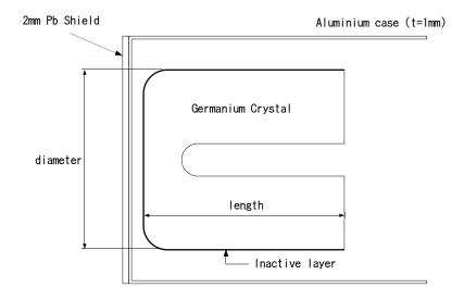
Figure 2.5: Internal structure of germanium detector.
