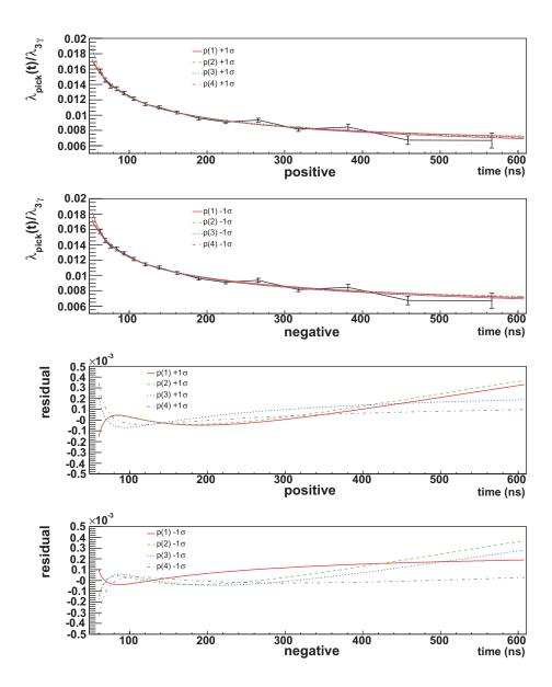
Figure 3.26: Uncertainties of the parameters (RUN II). The upper two figures are the deviated function when one parameter is fixed at  $+1 \sigma$  and at  $-1 \sigma$ . The lower two figures show the deviation of the pick-off ratio for each function.
