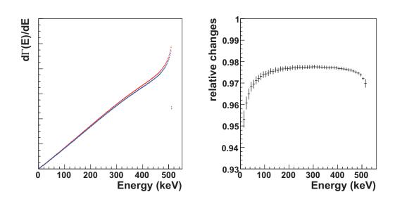
Figure 1.2: (a) The lowest order energy spectrum of  $3\gamma$  decay (red line) and the energy spectrum with the  $O(\alpha)$  correction (blue line). (b) The relative change of the energy spectrum by the  $O(\alpha)$  correction.
