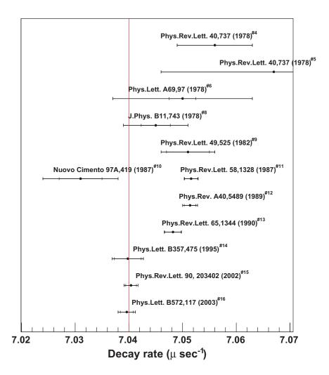
Figure 1.3: The chronology of the o-Ps decay rate measurement. The number on the right shoulder of each item indicates a corresponding index number in Table 1.4. Vertical band represents the  $O(\alpha^2)$ -corrected NRQED prediction of 7.039 979  $\mu s^{-1}$ . The inside line on each error bar represents a statistics error.
