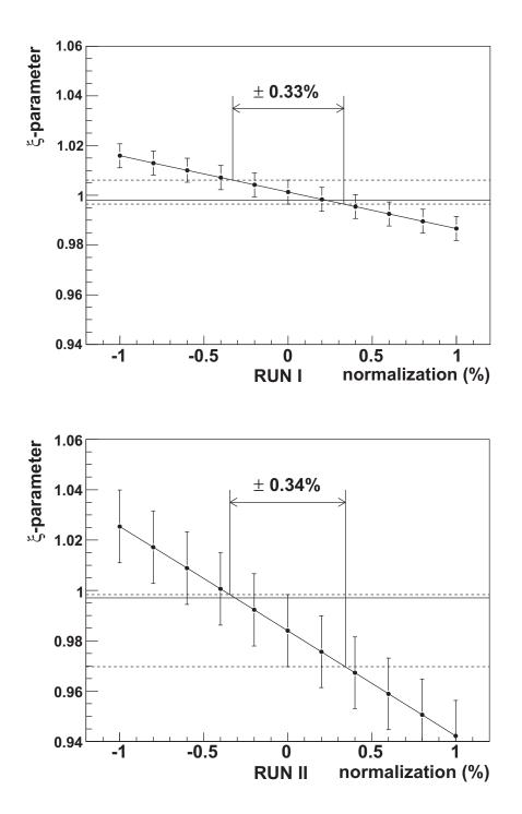
Figure 3.34:  $\xi$ -parameter with varied  $3\gamma$  normalization. The upper figure is the spectrum for RUN I and the lower figure is the spectrum for RUN II. The boundaries of the  $\pm 1 \sigma$  error from the  $\xi$ -parameter of the  $\pm 0.0 \%$ normalization is shown as dotted lines. This error corresponds to  $\pm 0.33 \%$ normalization for RUN I and  $\pm 0.34 \%$  normalization for RUN II. The  $\xi$ parameter of the prompt events is also shown as a solid line.
