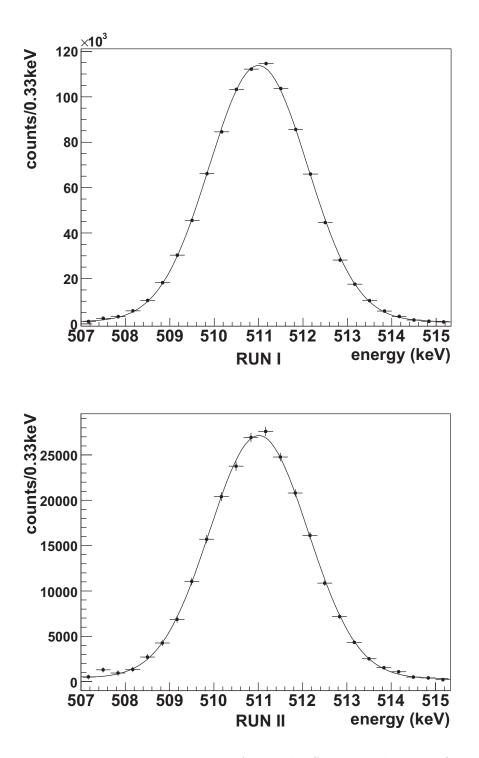
Figure 3.23: Energy spectrum of the pick-off events. The upper figure is the spectrum for RUN I and the lower figure is the spectrum for RUN II. The figure shows the spectrum after the subtraction of the  $3\gamma$  spectrum. The spectrum is a Doppler broadning  $2\gamma$  spectrum like the prompt events.
