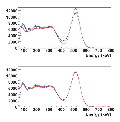
Figure 2.17: Comparison of the measured YAP spectrum with the simulation using <sup>85</sup>Sr source. The blue line is the measured spectrum and the red line is the spectrum generated by the Monte Carlo simulation. The difference is observed especially in the shape of photoelectric peak (the upper figure). The simulation with non-uniform photon collection efficiency reproduces the measured spectrum (the lower figure).
