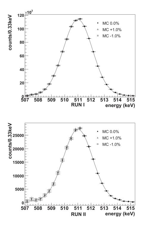
Figure 3.33: The pick-off spectrum with varied  $3\gamma$  normalization. The upper figure is the spectrum for RUN I and the lower figure is the spectrum for RUN II. The figure shows the pick-off spectra when the normalization of the  $3\gamma$  spectrum is varied by  $\pm 1$  %. The left side of the peak is shifted according to the variation of the normalization.
