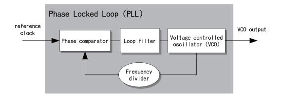
Figure 2.8: Schematic diagram of Phase Locked Loop (PLL).
