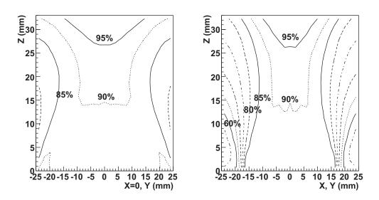
Figure 2.18: Collection efficiency of optical photon in YAP crystal. The left figure shows the collection efficiency along the Y axis on the center of crystal (X=0). The right figure shows the collection efficiency along the diagonal direction of X-Y plane. The photomultiplier is connected on the lower side of X-Y plane (Z=0).
