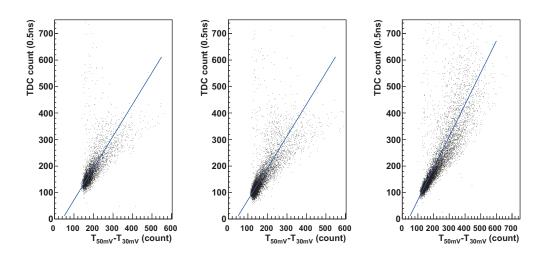
Figure 3.15: Time walk of the slow rise-time component. The detection time of the prompt events are plotted against the rise-time variable  $(T_{50 \ mV}-T_{30 \ mV})$ . Note that the small amount of  $3\gamma$  events are not rejected. The correlations are clearly seen in the figures. The linear function shown as the blue line is used to determin the time walk correction.
