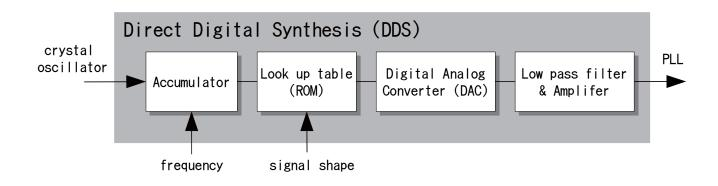
Figure 2.9: Schematic diagram of Direct Digital Synthesis (DDS)
