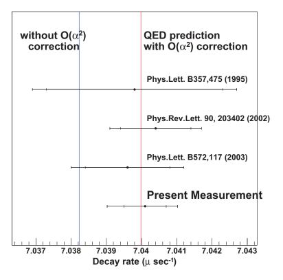
Figure 4.4: The relation between the resent measurements and the theoretical predictions. The red vertical line shows the  $O(\alpha^2)$ -corrected NRQED prediction of  $7.039\,979\mu s^{-1}$ . The blue vertical line shows the QED prediction without  $O(\alpha^2)$  correction, that is  $7.038\,226\mu s^{-1}$ .
