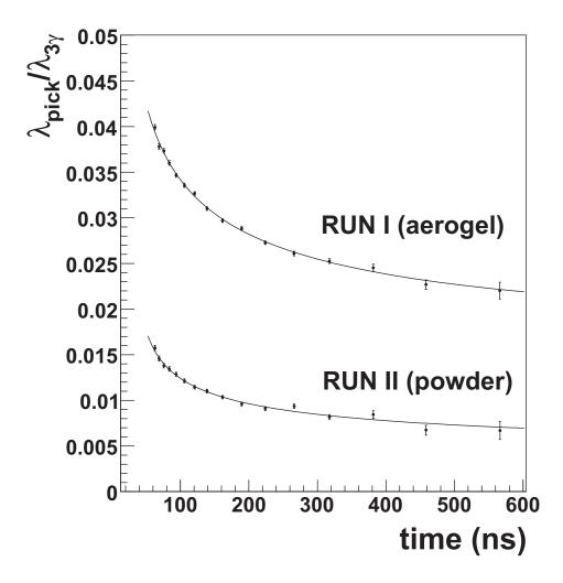
Figure 4.2: The measured pick-off ratios with two types of silica material. The pick-off ratio of silica aerogel is 3 times larger than that of silica powder.
