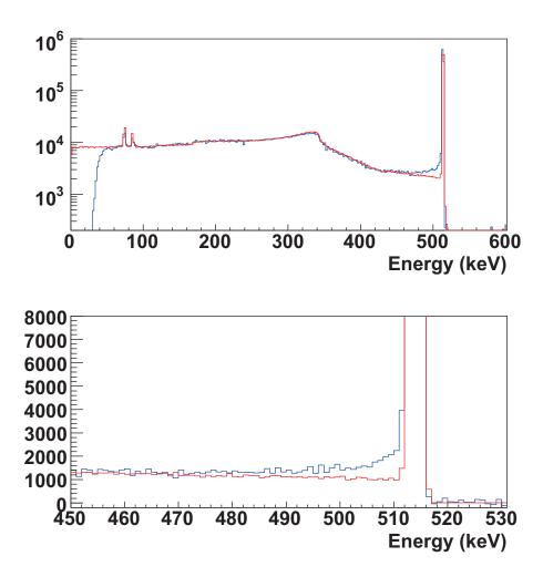
Figure 2.14: Comparison of the measured Ge spectrum with the simulation using <sup>85</sup>Sr source. The blue line is the measured spectrum and the red line is the spectrum generated by the Monte Carlo simulation. The two spectra are in good agreement with each other except for the region around the photoelectric peak. The lower figure is the enlarged spectrum around the photoelectric peak.
