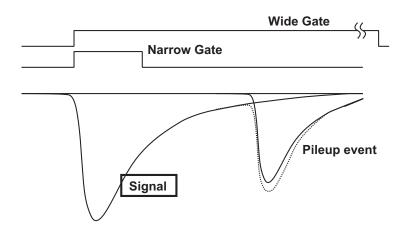
Figure 3.8: The schematic of the Narrow-Wide (NW) cut. The NW cut rejects the events where the succeeding signal diturbs the energy information of the preceding signal.
