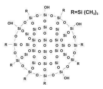
Figure A.1: Schematic diagram of  $SiO_2$  grain. Part of the surface functional groups are substituted, while there are still silanol groups left.
