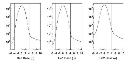
Figure 3.5: Base spectra for Ge detectors. The slow rise-time events are excluded in the figures. The events within  $\pm 4\sigma$  are selected. The two vertical lines in a figure show the boundaries of the cut.
