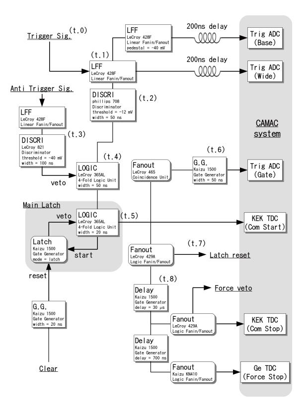
Figure 2.11: Schematic diagram of electronics for trigger system.
