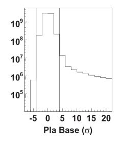
Figure 3.7: Base spectrum for the plastic scintillator. The events within  $\pm 4 \sigma$  are selected. The two vertical lines show the boundaries of the cut.
