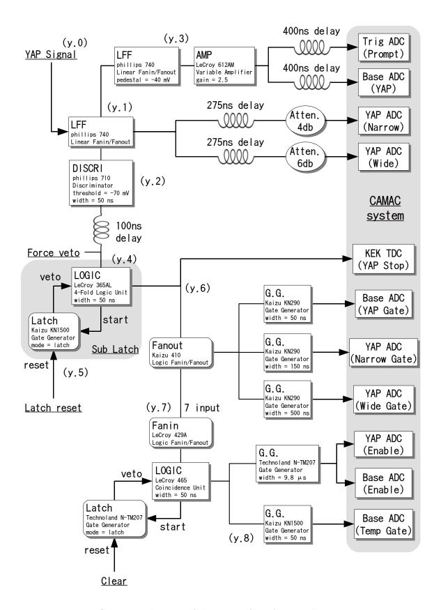
Figure 2.12: Schematic diagram of electronics for YAP scintillator system.
