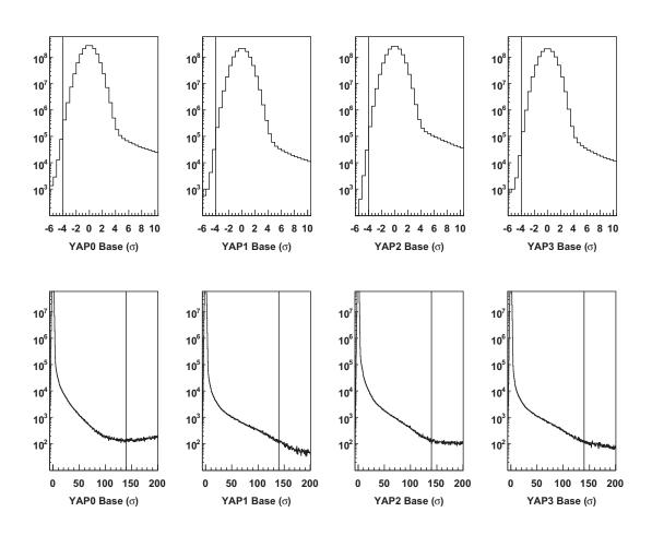
Figure 3.6: Base spectra for YAP scintillator. The events within the range from  $-4 \sigma$  to  $+140 \sigma$  are selected. The upper figures show the lower boundaries of the cut as the vertical line. The lower figures show the upper boundaries of the cut as the vertical line.
