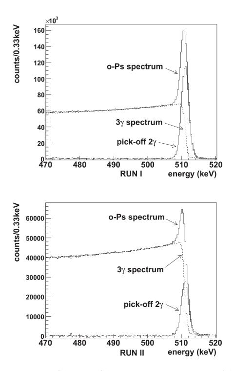
Figure 3.22: Subtraction of the  $3\gamma$  spectrum. Energy spectrum of the delayed region. The upper figure is the spectrum for RUN I and the lower figure is the spectrum for RUN II. The figure shows the spectrum after the subtraction of the accidental events. The  $3\gamma$  spectrum prepared by the simulation is normalized in the region from 480 keV to 505 keV. The difference is the contribution of the pick-off  $2\gamma$  events.
