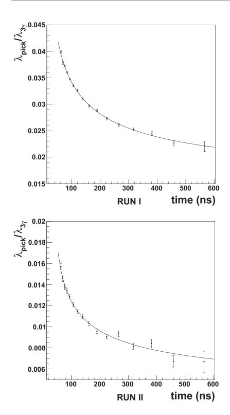
Figure 3.24: Pick-off ratio  $\lambda_{pick}(t)/\lambda_{3\gamma}$ . The upper figure is the spectrum for RUN I and the lower figure is the spectrum for RUN II. The slow curve represents the thermalization process of o-Ps. The pick-off ratio of the RUN I is about 3 times higher than the one of RUN II.
