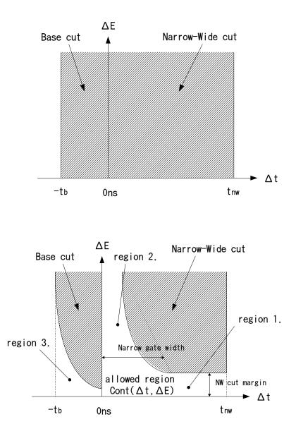
Figure B.4: Suppression region of the pile-up cuts. The upper figure shows the suppression region when the pile-up cuts are assumed to be perfect.  $\Delta E$  and  $\Delta t$  are the energy of the accidental signal and the time interval from the incident signal. The lower figure shows the suppression region in considering the energy dependence of the pile-up cuts. In this case, some regions are allowed.
