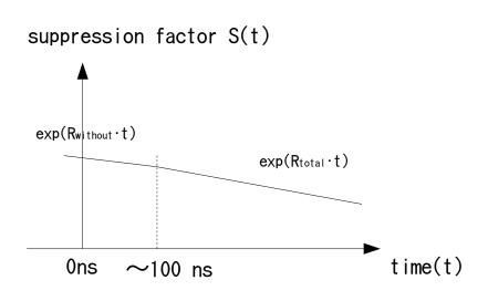
Figure B.6: Suppression factor S(t) for YAP scintillator. The events in the later region are suppressed by the first hit condition.
