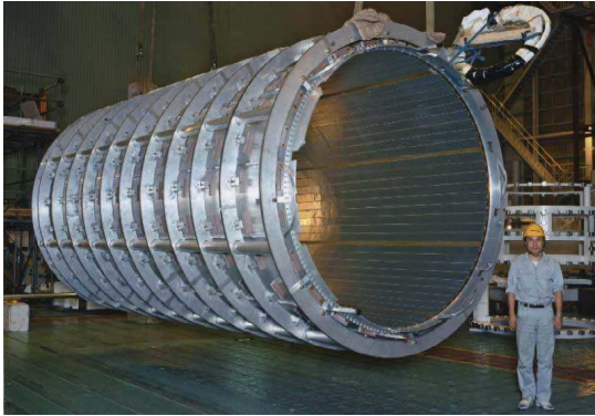
Figure 2.6: The central solenoid magnet of ATLAS.
