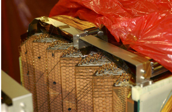
Figure 2.21: A cross section of LAr electromagnetic calorimeter.
