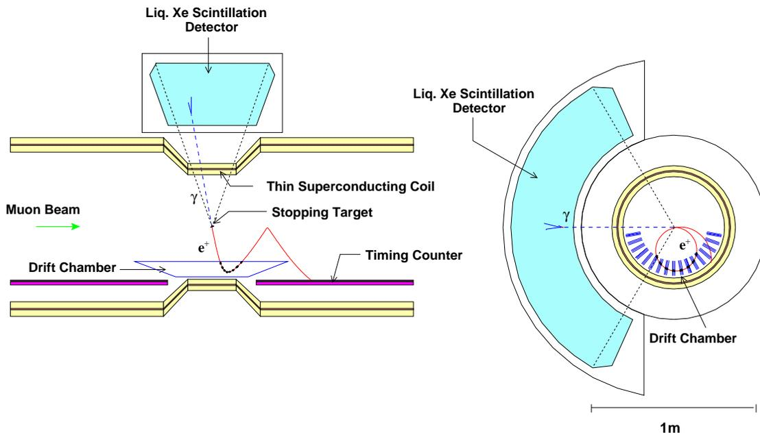
Figure 2. Detection of a  $\mu \rightarrow e\gamma$  event in the PSI experiment
