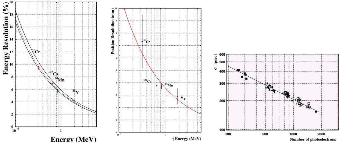
Figure 4. Energy, position, and timing resolutions (from left to right) as a function of energy or photoelectron statistics, obtained by the small prototype.
