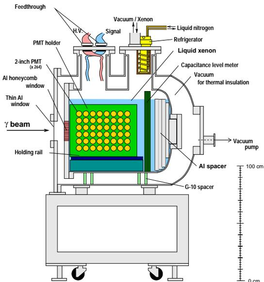
Figure 5. Large Prototype Xenon Detector
