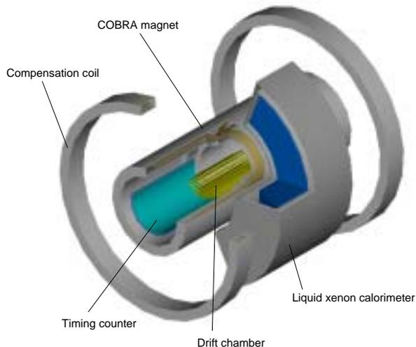
Figure 1. An experimental set-up of the new PSI experiment
