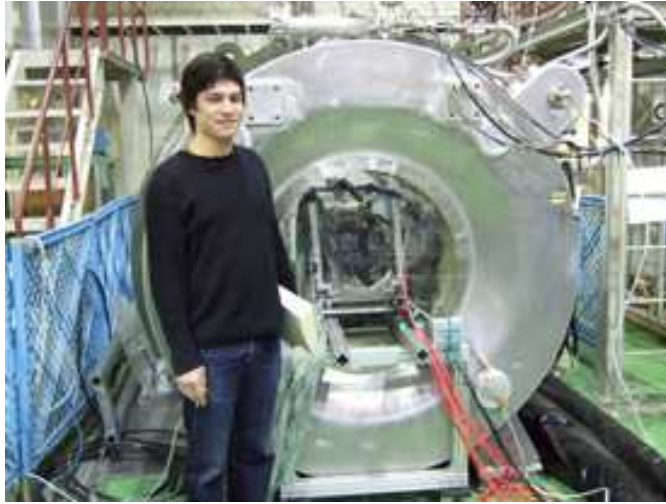
FIGURE 7. Superconducting magnet: Bore size is 80 cm and the uniform magnetic field can be applied up to 1T.
