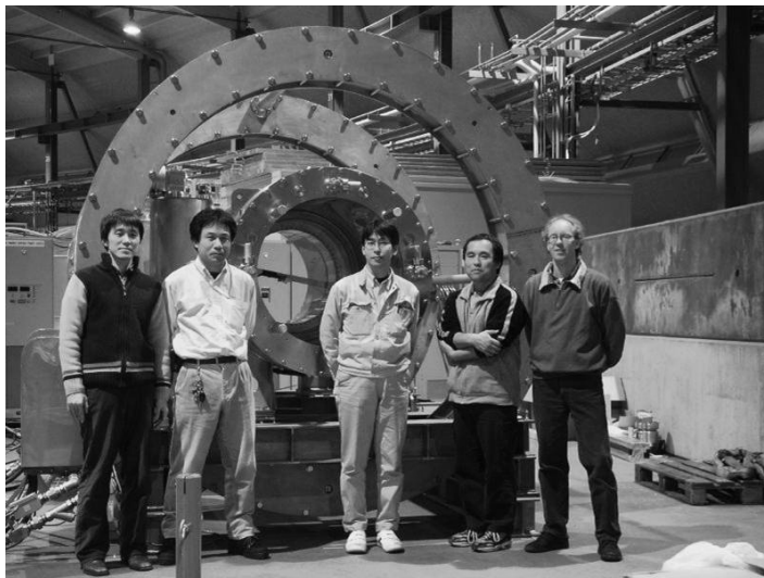
Figure 2: The COBRA magnet operating at PSI. The large Helmholtz coils seen in the figure are to compensate the magnetic field at the gamma ray detector down to below 50 Gauss.
