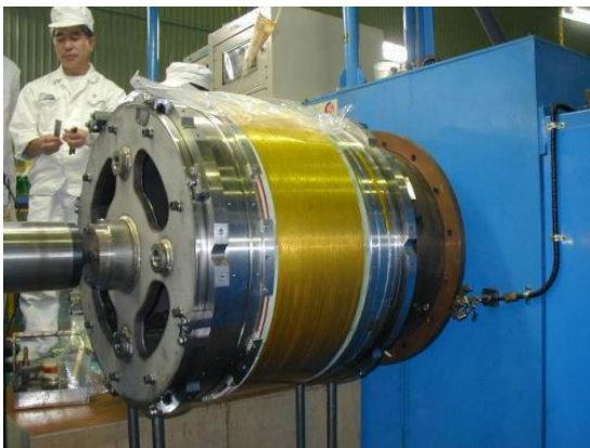
Figure 2. The central coil of the COBRA magnet is being wound.
