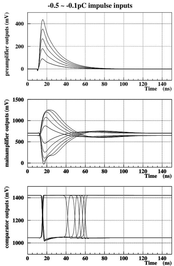
Figure 4: PSPICE simulations of the preamplifier, main-amplifier and comparator outputs.
