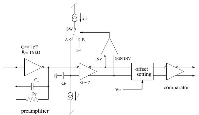
Figure 1 : Block diagram of the ASD chip.
