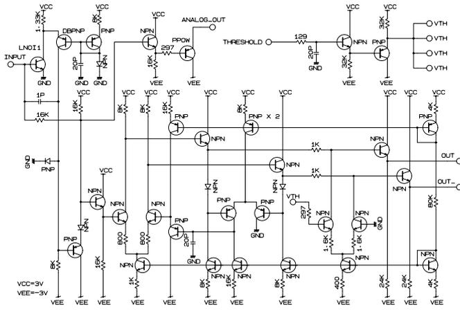
Figure 2 : Preamplifier, baseline restorer and main-amplifier schematics.
