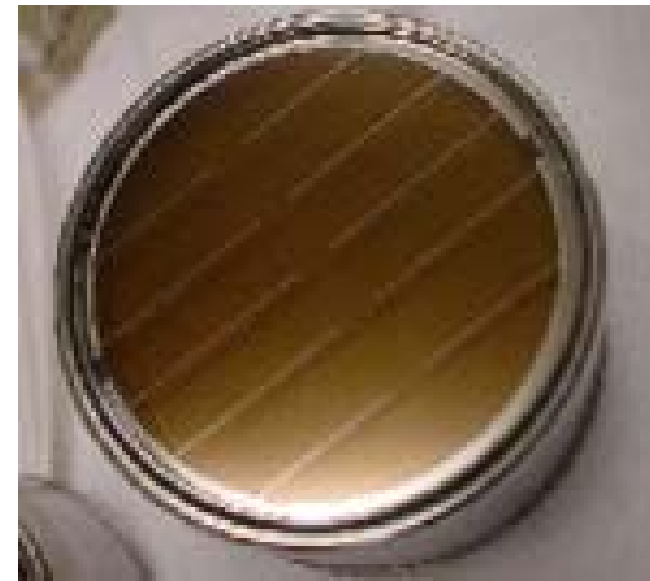
Hamamatsu R9288 photocathode: K-Cs-Sb Aluminum strip Q.E. improved
