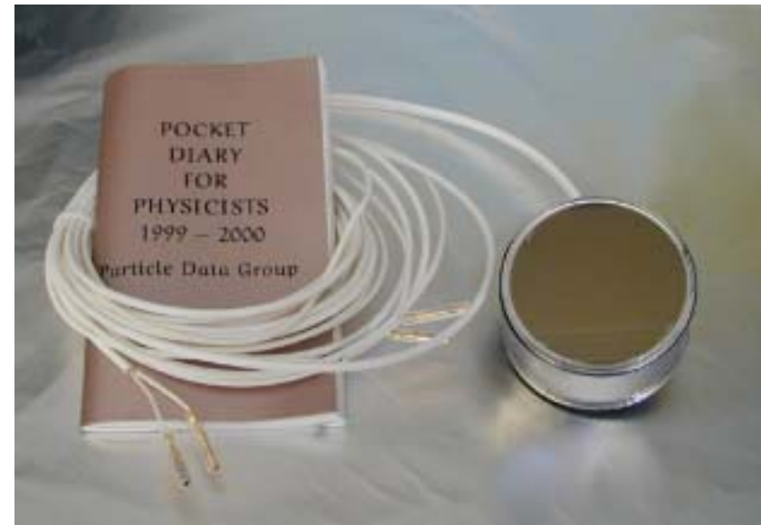
Hamamatsu R6041 photocathode: Rb-Cs-Sb Q.E. : ~10% Installed in Large Prototype
