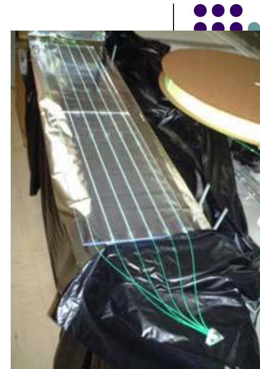
Top View of Prototype Scintillators with linear grooves
