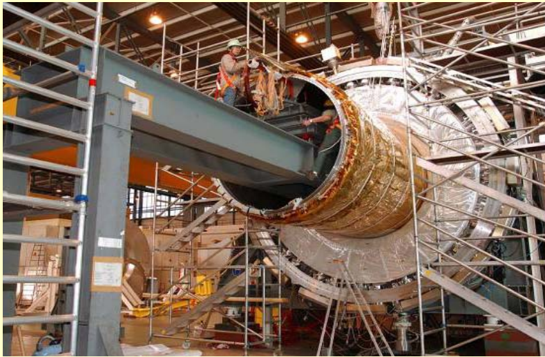
Insertion of the solenoid in the calorimeter cryostat (Japan-ATLAS contribution)
