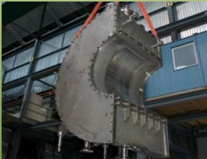
Liquid Xenon Scintillation Detector (gamma)
