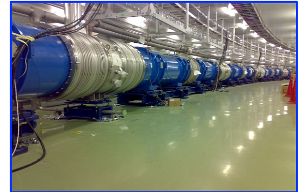
Bend the beam by ~80° Using Super-conducting combined function Magnets
