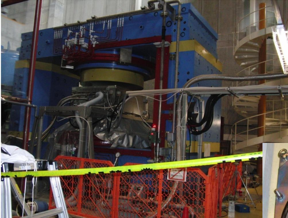
The MA core is treated inside a high-temperature large furnace, which is located inside the magnet gap.
