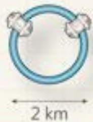
TEVATRON 1985-present Accelerates: Protons Energy: 1 TeV
