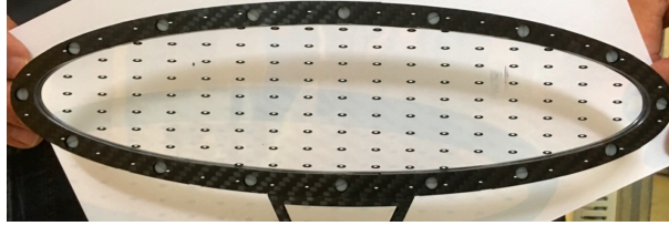
Figure 3.20: The muon stopping target in the MEG II experiment[27]. Optical markings are printed on the scintillator target.
