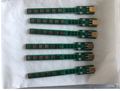
Figure 5.3: A picture of new SiPMs soldered onto PCBs.
