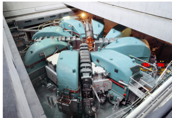
Figure 3.18: The 590 MeV ring cyclotron [30].
