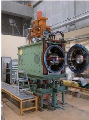
Figure 6.6: Picture of the electrostatic separator (*ESS*) before installation. The *ESS* is one of the essential elements for the beamline to extract a clean  $K^+$  beam.
