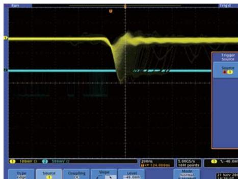
Figure 3.9: Typical chamber raw signal. It had an overshoot and some ringing.
