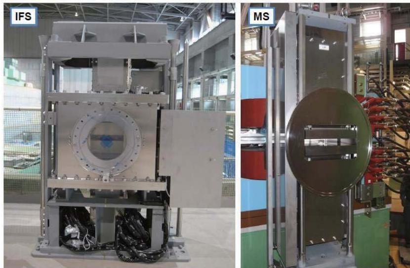
Figure 6.4: Picture of the intermediate focusing slits ( $IFX + IFY$ ) and the mass slit ( $MS$ ) before installation. Both slits are located at the vertical focusing point. The  $IFY$ , in particular, has a crucial role for the removal of pions in spite of the use of a single stage separator. In addition,  $IFX$  is useful to control the overall beam acceptance.
