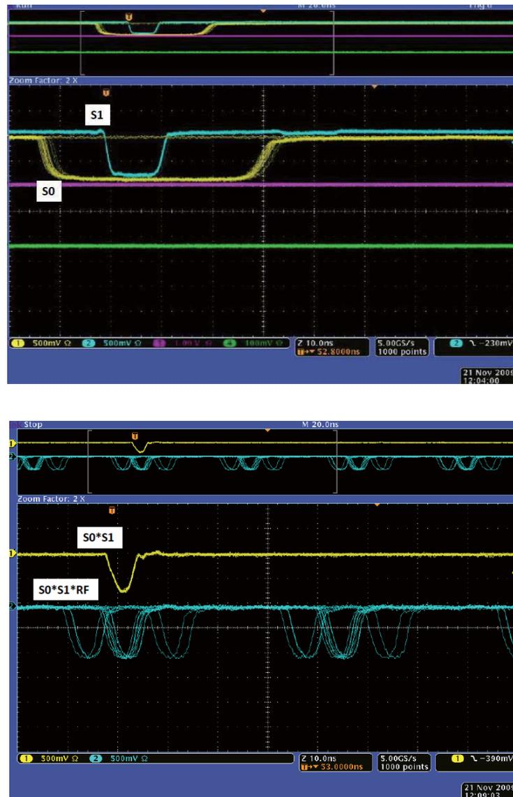
Figure 3.5: Pictures of oscilloscope. The top one shows the S0 and the S1 counter signal which correspond to the yellow line and the blue line, respectively. The S1 counter signals appear 10 ns later than the S0 signals. On the other hand, the bottom one shows the  $S0 \otimes S1$  and  $S0 \otimes S1 \otimes RF$  corresponding to the yellow line and the blue line, respectively.  $S1 \otimes RF$  coincidence signal has 3 components due to the three kinds of positive charged particles.
