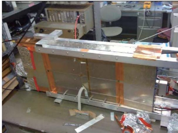
Figure 2.5: Picture of 1/5 prototype polarimeter
