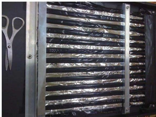
Figure 6.9: Picture of the beam Hodoscope. The Hodoscope is composed of 24 scintillators with a thickness of 12 mm in a stainless steel frame.
