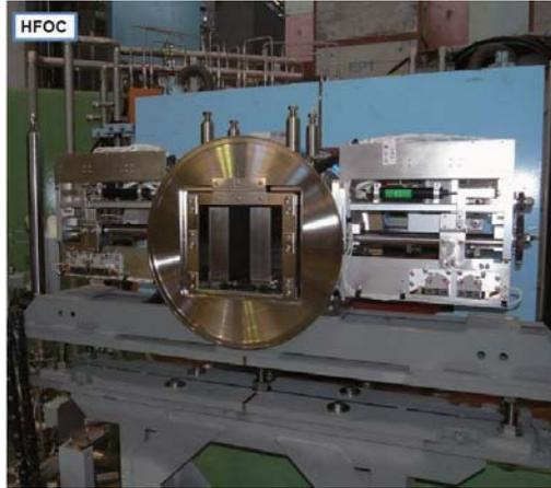
Figure 6.5: Picture of the horizontal focusing slit (*HFOC*) before installation. The *HFOC* is placed before the final doublet  $Q7 - Q8$  and is also useful for the removal of the pion contamination in the beam.
