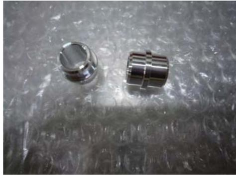
Figure 5.11: Tube to template connector.
