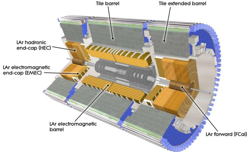
Figure 3.5: An overview of the ATLAS calorimeter system [58]. The calorimeter covers  $|\eta| < 4.9$  using different types of modules. The electromagnetic calorimeters are surrounded by the hadronic calorimeters.
