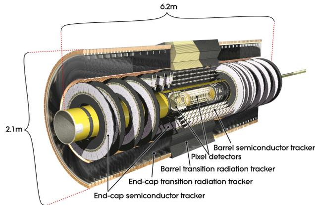
Figure 3.3: An illustration of the Inner Detector [58]. Both barrel and endcap regions are shown.
