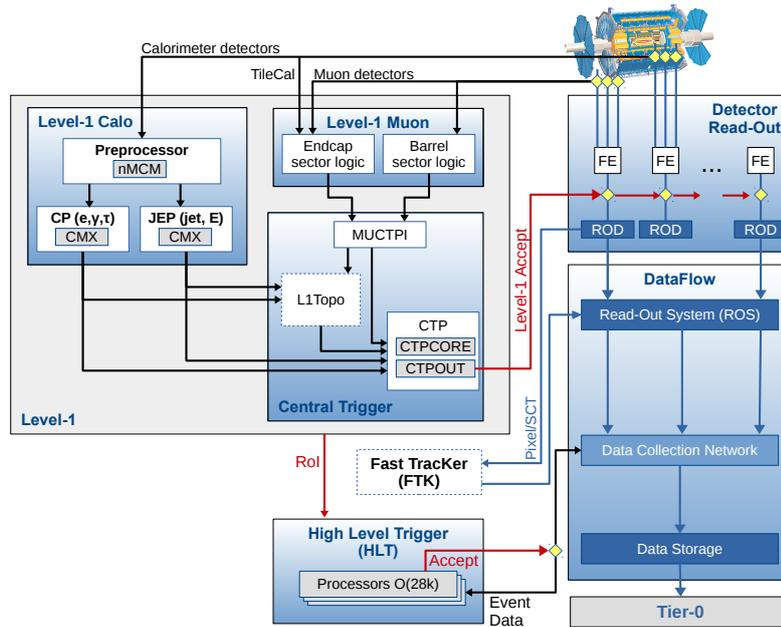
Figure 3.8: The ATLAS trigger and data acquisition system [62]. The trigger system consists of two stages: Level-1 and HLT. The hardware-based Level-1 trigger uses information from the calorimeter and muon detectors, and issues Level-1 Accept and provides region of interest (ROI) information to the HLT. The software-based HLT issues final accept signals to record events using offline-like reconstruction algorithms.
