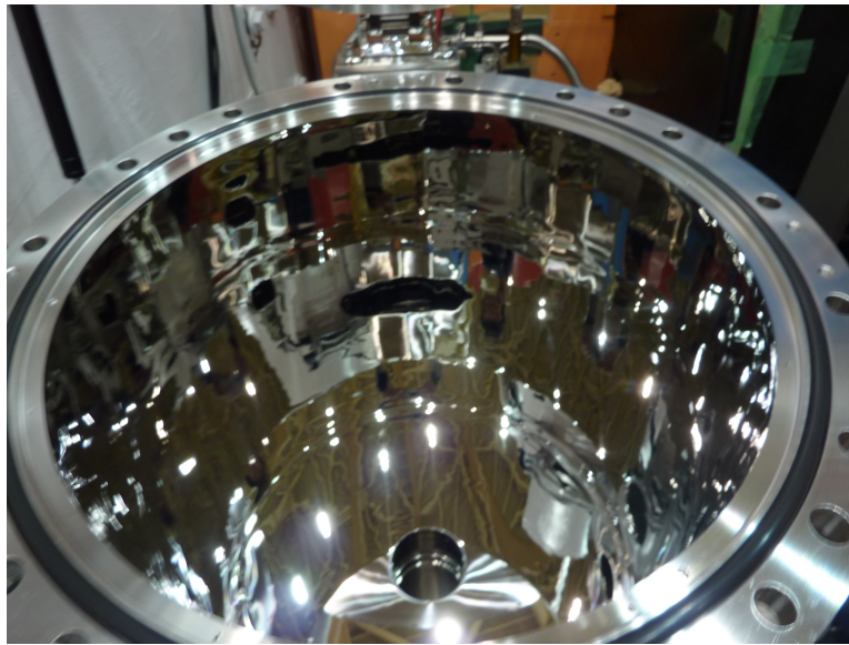
Figure.6.9 Photograph of the inside of the storage container. The upper lid of the storage container was opened, the test material was removed, and the picture was taken from above. The inner surface is subjected to the composite electrolytic polishing treatment and the inner surface is lustered like a mirror.
