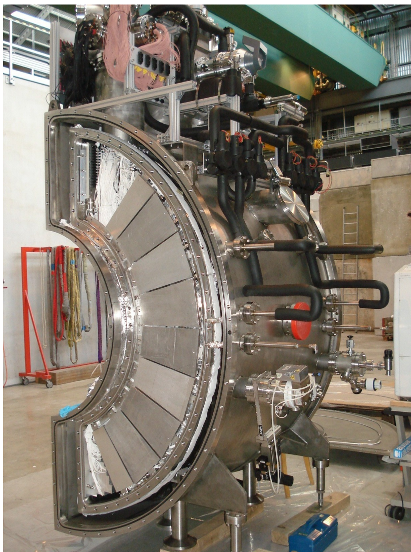
Figure 3.27: Picture of LXe gamma-ray detector. It was just before closing covers. All components were mounted.
