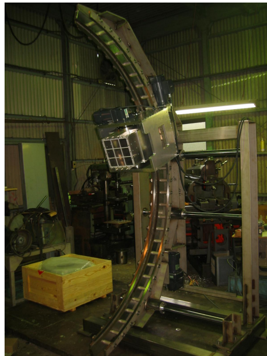
Figure 3.40: Movable stage of the NaI detector to be placed at the opposite side of the LXe gamma-ray detector.
