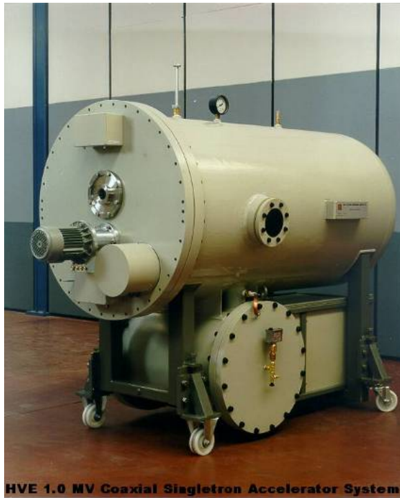
Figure 3.41: 1 MeV Cockcroft-Walton proton accelerator.
