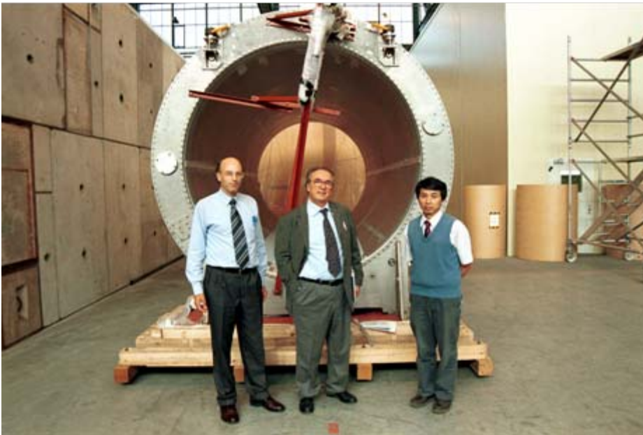
s.c. solenoid (Sep.2001) already integrated with barrel LAr and brought into the pit
