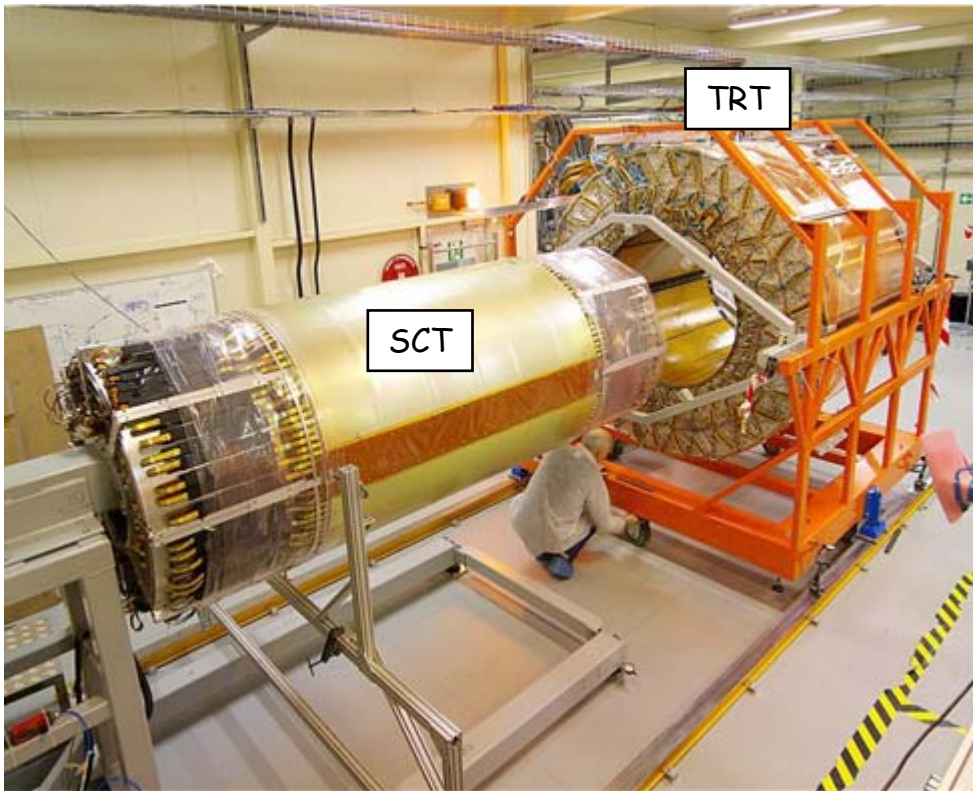
Barrel Si detector(SCT) was inserted into barrel TRT in Feb. 2006.
