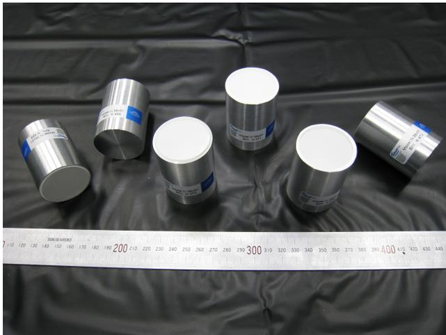
Figure 3.20:  $\text{LaBr}_3(\text{Ce})$  scintillators.Table 3.2: Properties of  $\text{LaBr}_3(\text{Ce})$  [66]. The properties of  $\text{NaI}(\text{Tl})$  are also listed for comparisons.
