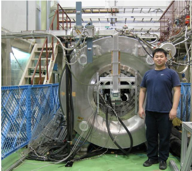
(a) Large bore superconducting magnet.
