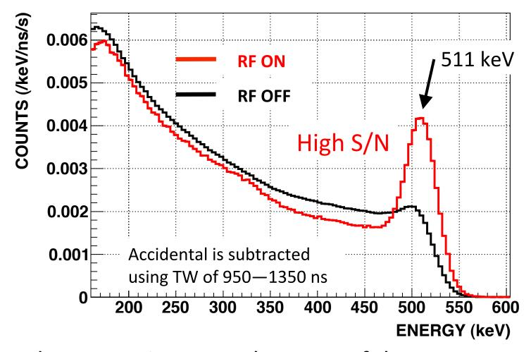
2γ decay rate increases because of the Zeeman transition. Zeeman transition probability is calculated from the difference between RF-ON and RF-OFF.
