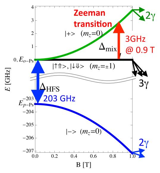
When a microwave field with a frequency of  $\Delta_{\text{mix}}$  is applied, transitions between the  $m_z$ =0 and  $m_z$ =±1 states of o-Ps are induced.
