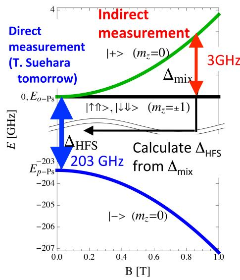
In a static magnetic field, the p-Ps state mixes with the  $m_z$ =0 state of o-Ps (Annihilate into 2  $\gamma$ -rays).
